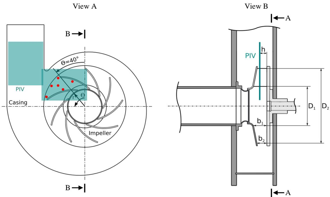
Figure 5: Position of the PIV measurement planes and probe points for the statistical significance (red dots)
