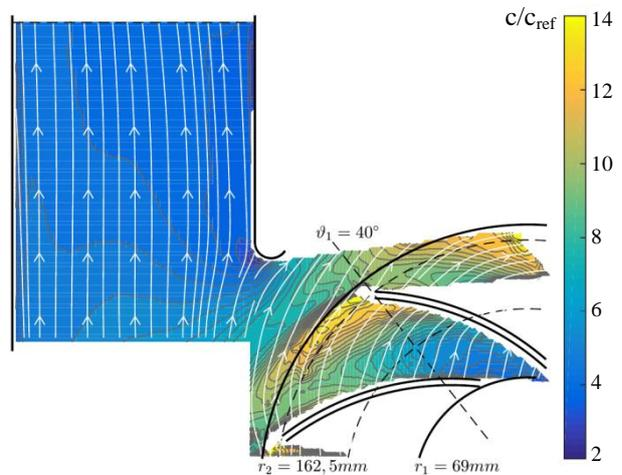
Figure 7: Normalized absolute velocity at M3
