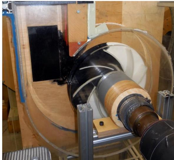
Figure 2: The model fan in the spiral casing
