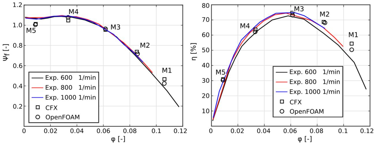
Figure 4: Pressure head and efficiency of the fan conducted from measurements at different rotational speeds and from numerical simulations
