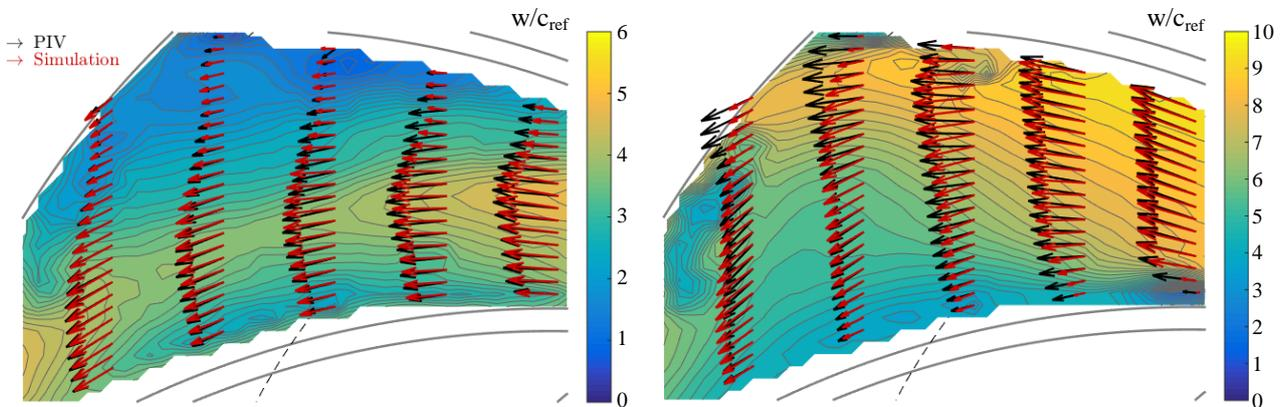
Figure 10: Normalized relative velocity as contour plot and comparison of measurement and numerical simulation (OpenFOAM®) by means of velocity vectors at M3 (left) and M1 (right)
