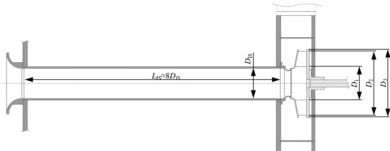
Figure 3: Inlet section, suction nozzle and impeller
