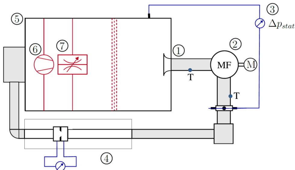
Figure 1: Test loop; 1- inlet section, 2- model fan, 3 – measurement of pressure difference, 4 – measurement of volume flow rate, 5 – settling chamber (with screens for flow homogenization), 6 – booster fan, 7 – throttle, MF – model fan, M - motor
