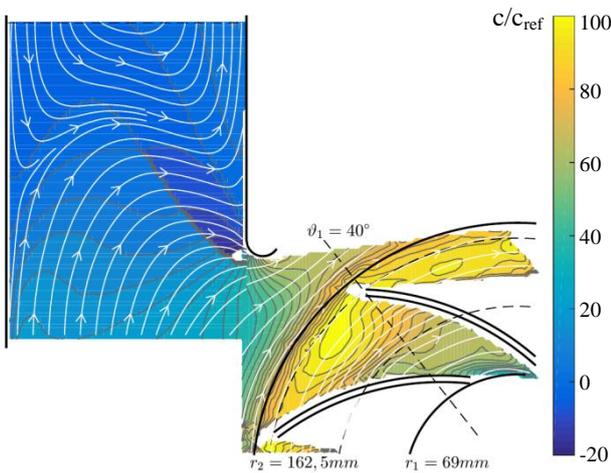
Figure 8: Normalized absolute velocity at M5
