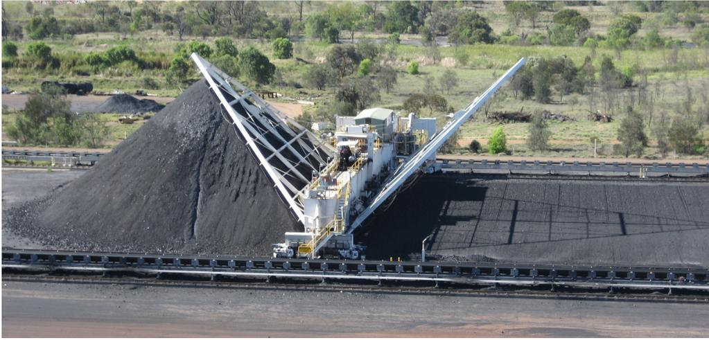
Figure 2.5: Photo on a railed reclaiming machine at a longitudinal blending bed
