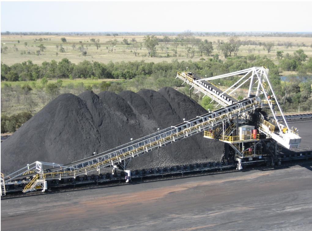
Figure 2.4: Photo of a railed stacking machine at a longitudinal blending bed
