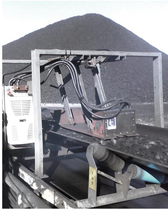
Figure 2.1: An online X-ray fluorescence analyzer mounted on a sled gliding over coal on a conveyor belt
