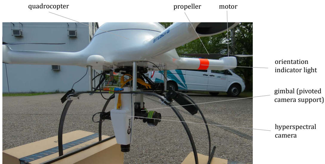
FIGURE 2.2: Prototypical UAV system and hyperspectral camera. Source: Bodo Bernsdorf, EFTAS Fernerkundung Technologietransfer GmbH.
