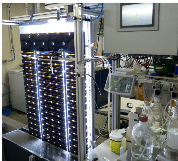
Figure 1. Flat-panel airlift photobioreactor (30 L) with artificial illumination and SPS control unit used for the cultivation of P. tricornutum at Fraunhofer IGB, Stuttgart.
