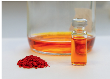
Figure 2. EPA- and fucoxanthin-rich lipid fraction (right) extracted by PLE and purified fucoxanthin powder (>90 wt %) (left).
