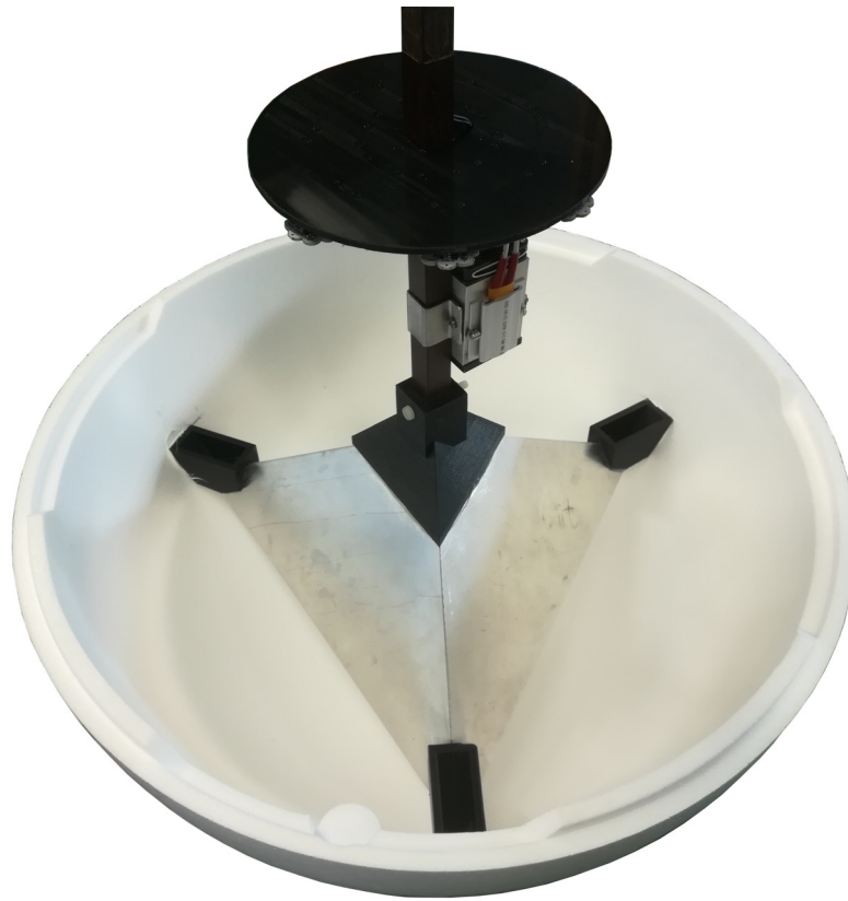
Figure 4.2: One half of the Styrofoam sphere with the metal corner reflector attached to it. Additionally, a heater and LEDs are placed inside the sphere.
