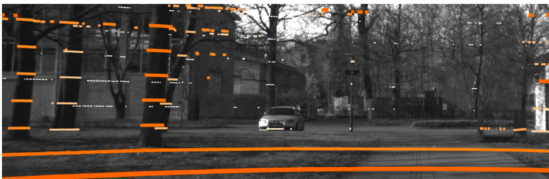
Figure 10.11: Grayscale camera image with projected measurements of a LiDAR after calibration. The color and size of the markers encode the range. An assessment of the camera to LiDAR calibration is possible based on the overlap of projected LiDAR measurements and the image at characteristic objects such as trees and poles.
