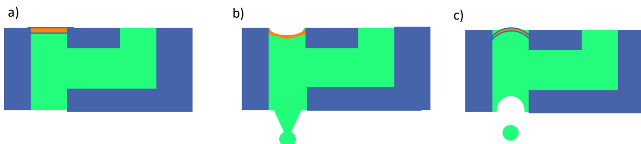
Figure 5.4: representation of ink droplet generation inside the printhead. In orange the piezoelectric component, in green the ink solution and in blue the walls of the printhead. Panel a) the piezoelectric element is in the idle configuration no ink is released. Panel b) the piezoelectric element receives the voltage impulse, changes its configuration inducing a pressure in the ink, and starts to produce the droplet. Panel c) the piezoelectric elements returning to its starting position is removing the pressure and the droplet is released.
