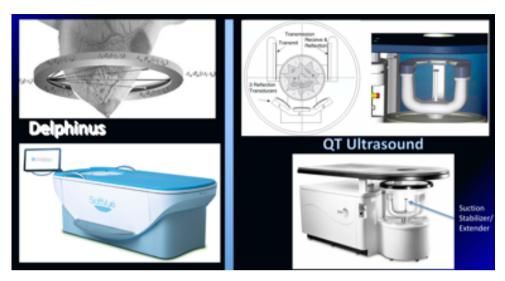
Figure 11: Two commercially available UTT systems. Left: Delphinus SoftVue [31] system with 2048 element ring array operating at up to 2.5 MHz; Right: QT Ultrasound's system with a large, planar transmitter, a 1536 element transmitter and receiver array operating at 0.3 to 1.3 MHz and three conventional curved linear arrays conventional pulse echo imaging [32].
