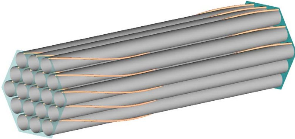
*Figure 1: Configuration of 19-rod bundle with wrapped wires*
