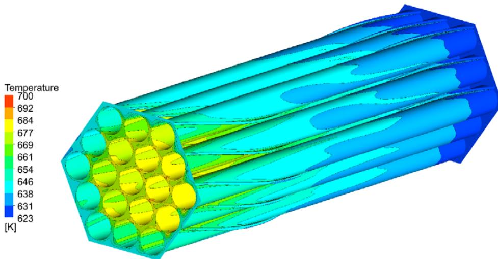
Figure 5: 19-rod bundle temperature distributions
