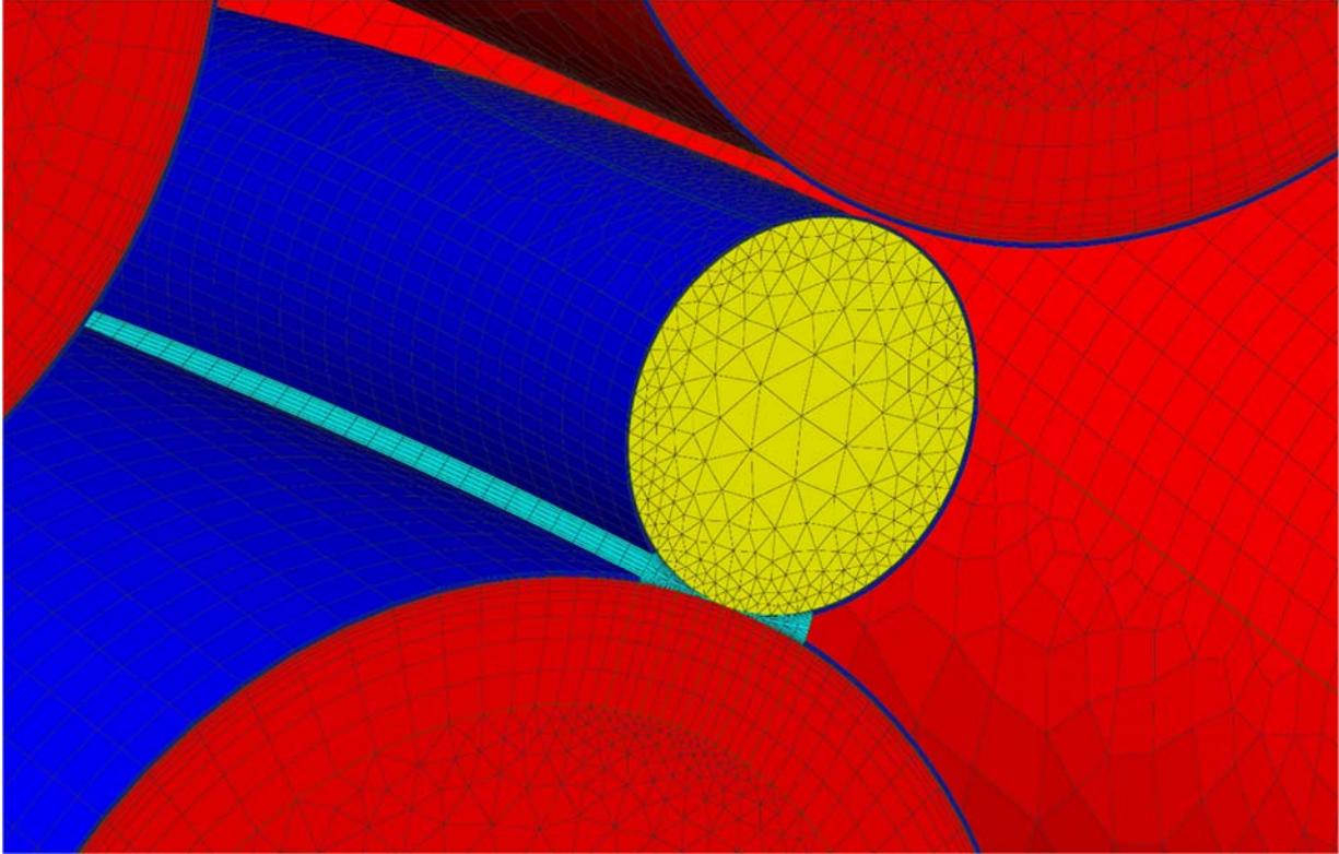
*Figure 2: Contact area modeled with spiral extrusion block*
