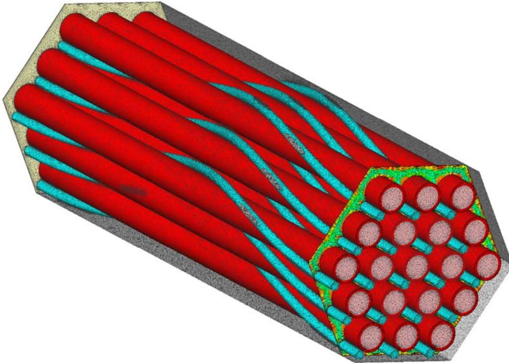
Figure 4: 107 million cell high-quality mesh of the 19-rod bundle
