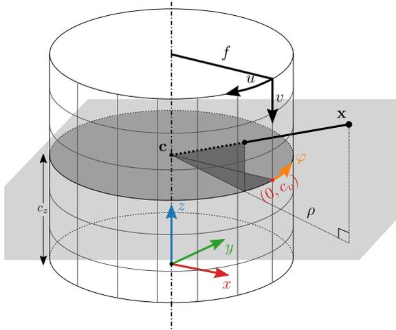
Figure 4.3: Cylindrical projection model used for a rotating LiDAR.
