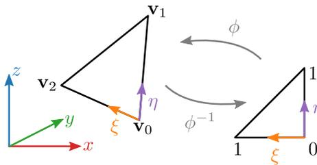
Figure 6.7: Mapping from an arbitrary triangle to the unit triangle and back.
