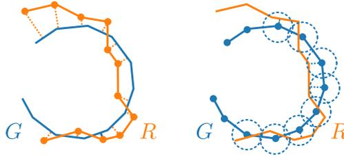
Figure 7.4: Error metrics from [SCD<sup>+</sup>06] to compare a reconstructed mesh (R) with a ground truth mesh (G). Definition of accuracy on the left side and completeness on the right. For the completeness metric, the inlier distance  $d$  is shown as dashed circles.
