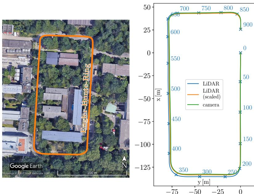
Figure 8.2: Test route on Engler-Bunte-Ring in Karlsruhe, Germany (left) and trajectories from localization (right). Scale and orientation of both images are intentionally not the same. Frame numbers are plotted every 50 frames. The frame rate is 10 Hz.
