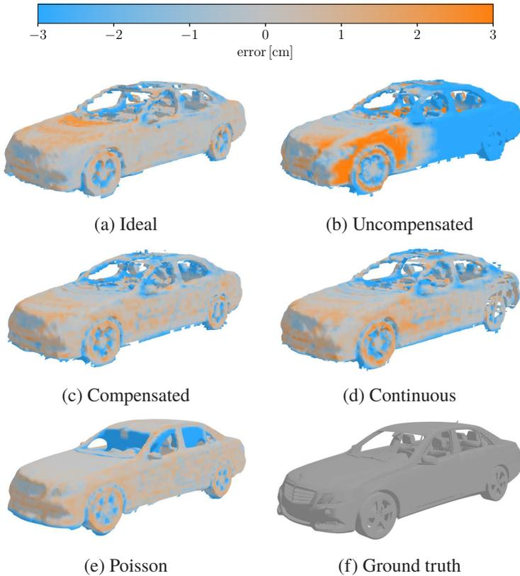
Figure 7.5: Signed distance of the reconstructed surface to the ground truth. Errors are cut off at 3 cm for better visualization. Negative values indicate that the reconstruction is too small, positive values indicate that it is too large.
