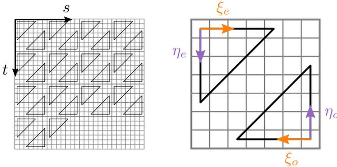
Figure 6.5: Grid structure of the texture map (left) and local coordinate systems of one of its tiles (right).
