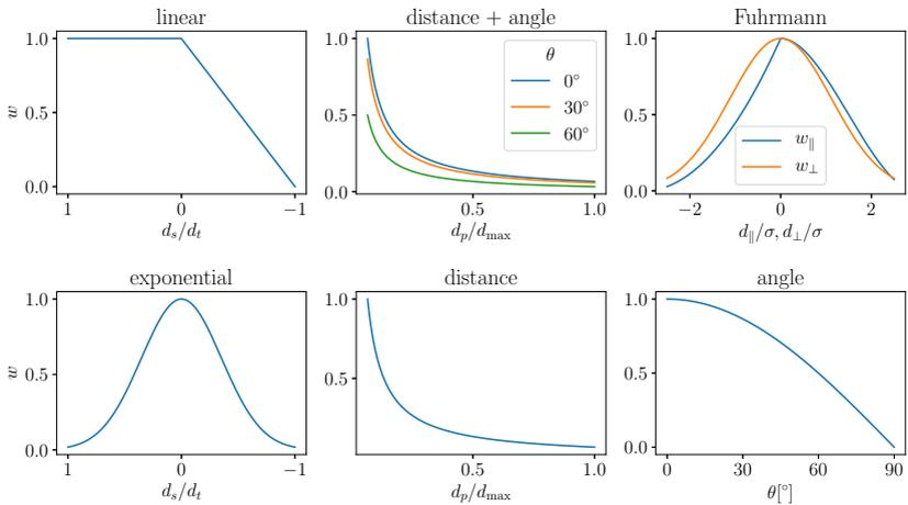
Figure 4.8: Overview of different weighting schemes used in literature. The weights in the left column depend on the signed distance estimate  $d_s$ . The weights in the center column depend on the distance of the measurement. Fuhrmann weights depend on the parallel and orthogonal distance with respect to the surface normal.  $\theta$  denotes the angle between line of sight and surface normal.
