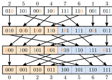
Figure 3.15: Radix sort using binary representation of the values zero to seven. In each iteration (row) the value of the highlighted digit determines the partial sequence it is moved to (light shaded boxes).
