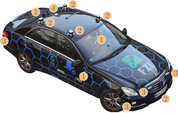
Figure 8.1: Image of our experimental vehicle Bertha. It is equipped with numerous different sensors, such as color and monochrome cameras behind the windshield, the rear window and below the side mirrors (1), four LiDAR sensors with 16 scan lines each on the top of the car and one four line scanner in the front bumper (2), full coverage of the surrounding by radars (3), and GPS (4). Not visible are the wheel encoders which provide wheel odometry and an IMU for acceleration and turn rates.
