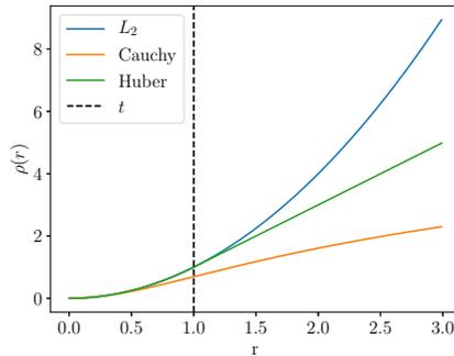
Figure 3.17: Overview of different loss functions. The threshold for all methods is set to  $t = 1$ .
