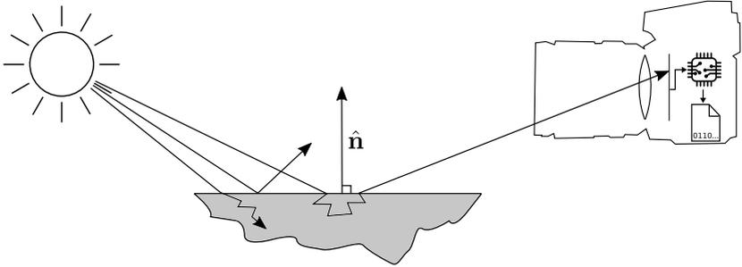
Figure 3.5: Image formation process from light source to digital image.
