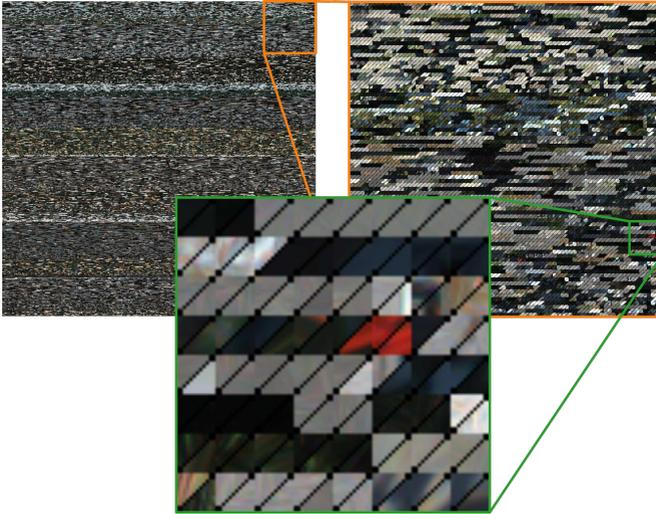
Figure 6.6: Real texture map example of size  $5772 \times 5772$  px (top left) and successively enlarged areas (orange, green rectangles) showing the map's layout up to the individual texels.
