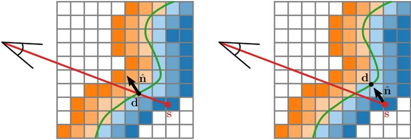
Figure 4.4: Two possible ways to determine the destination point  $\mathbf{d}$  for a given source point  $\mathbf{s}$ . Orange represents positive and blue represents negative values of the TSDF. On the left,  $\mathbf{d}$  is determined by finding the zero crossing along the red line. On the right,  $\mathbf{d}$  is determined by moving along the normal in  $\mathbf{s}$  by a distance equal to the signed distance value in  $\mathbf{s}$ .
