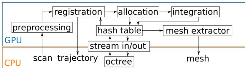
Figure 4.1: Overview of the reconstruction pipeline.
