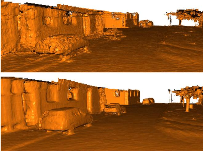
Figure 5.3: Area which was passed three times during recording. Reconstruction from misaligned chunk poses (top) and after three iterations of pose refinement (bottom).
