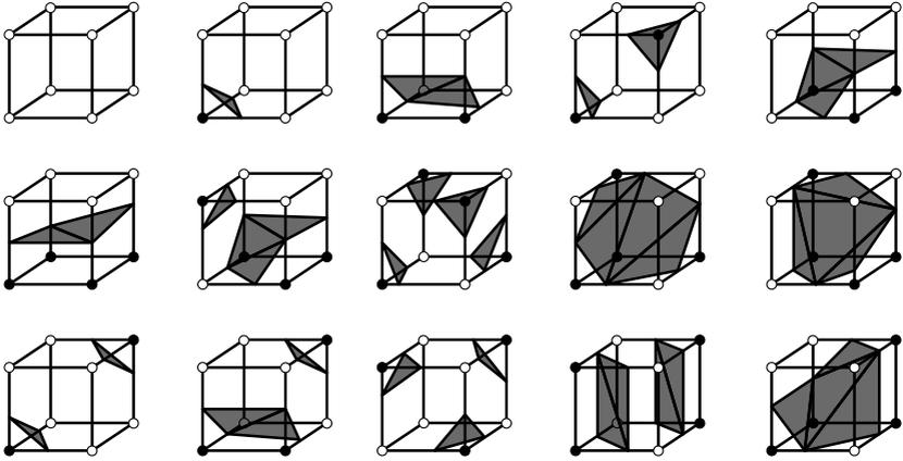
Figure 4.9: All possible constellations that can appear. Filled and empty circles in the corners of the cubes indicate opposite signs of signed distance values.
