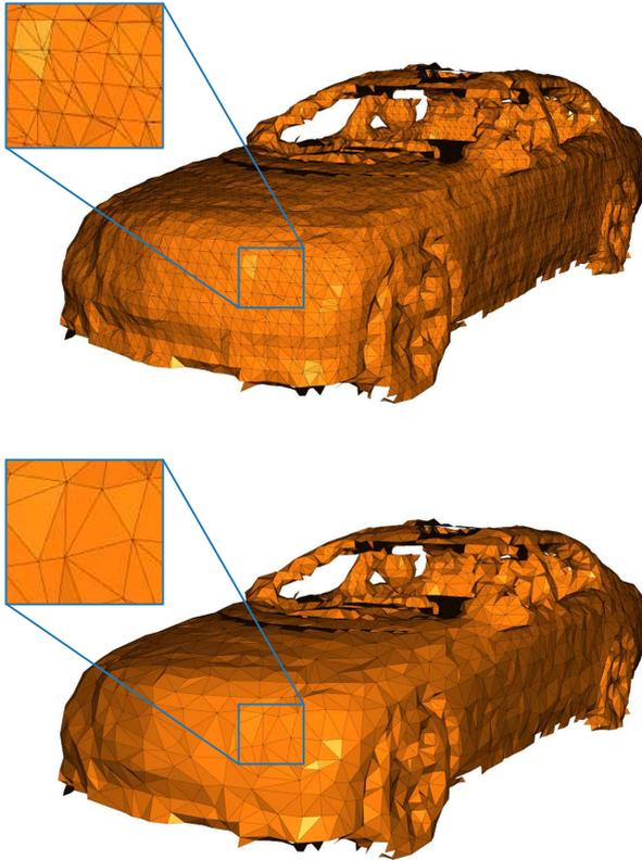
Figure 4.10: Mesh simplification of a reconstructed car. Original mesh (top) and simplified mesh with the number of faces reduced to 30 % (bottom).
