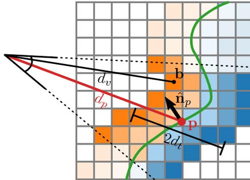
Figure 4.7: Updating the signed distance field for a single pixel of a sensor. All voxels are projected into the sensor model. Those voxels that fall into a pixel and lie within the truncation distance (highlighted cells) are updated with the corresponding measurement  $\mathbf{p}$ .
