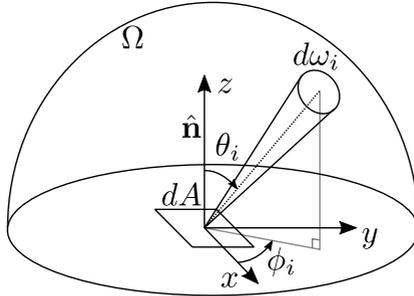
Figure 3.4: Illumination of a surface patch from a single direction.
