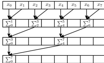
Figure 3.16: Summing up all elements of an array using reduction.
