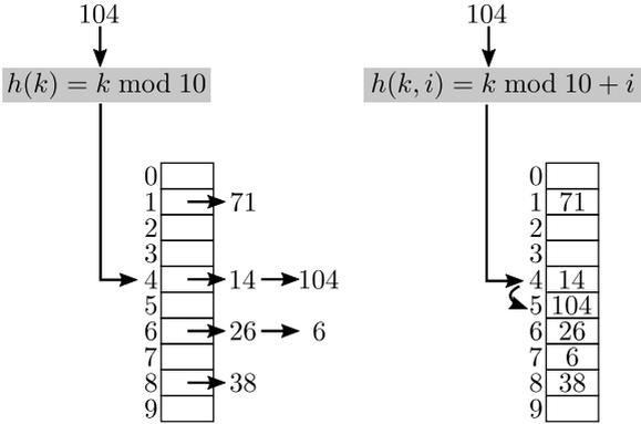
Figure 3.11: Two strategies to resolve hash collisions. Left: Hash table using linked lists. Entries which hash to an occupied entry are appended to the list. Right: Hash table using probing. When a collision occurs, the hash value is recomputed increasing  $i$  by one until a free entry is found.
