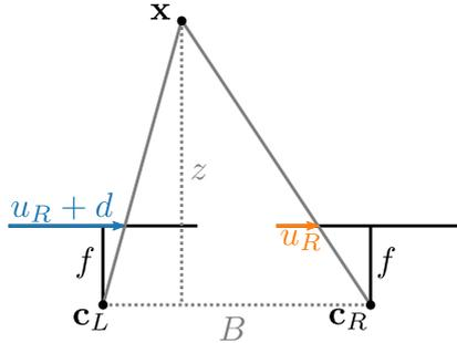
Figure 3.7: Depth computation from disparity  $d$ .
