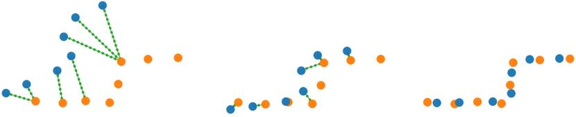
Figure 3.18: A source point cloud (blue) is aligned to a destination point cloud (orange) using nearest points as correspondences (dashed green lines). After two iterations (from left to right) both surfaces match. In each iteration, the distances between corresponding points are minimized.
