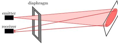
Figure 3.6: Diaphragm filtering out ambient light. The returned light comes from the footprint of the laser beam on a surface, and therefore can have different run times, as shown by the two dashed lines.
