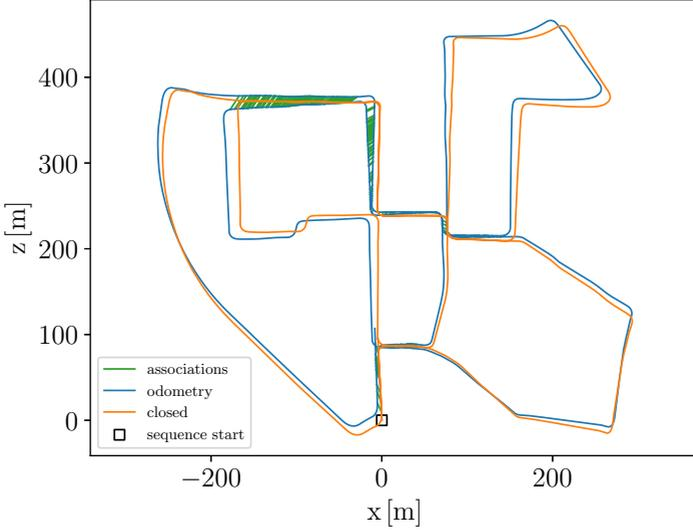
Figure 5.2: Trajectory before (blue) and after loop closure (orange). The green lines connect corresponding poses from the loop closure detection step.
