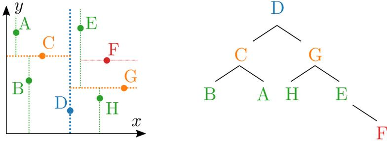
Figure 3.9: Left: Partitioning hyperplanes. The line thickness represents their depth in the tree (the thinner, the deeper). Right: Corresponding tree structure.
