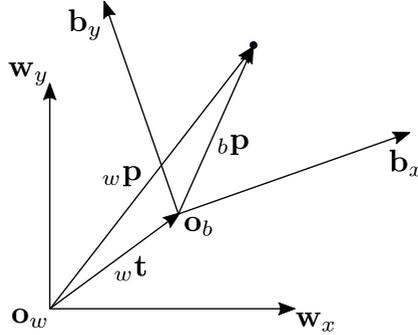
Figure 3.3: Visualization of point coordinates of the same point  $\mathbf{p}$  in two coordinate systems  $B$  and  $W$ .
