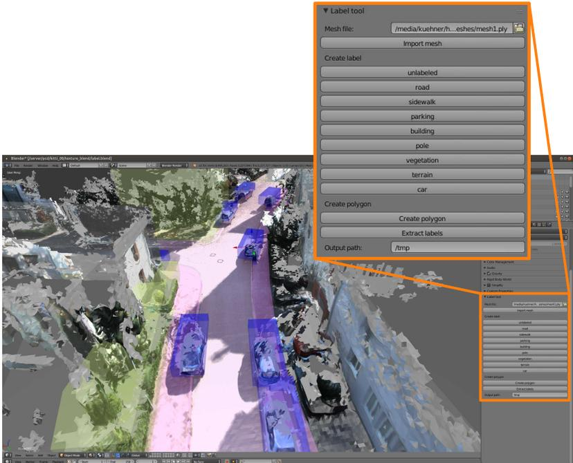
Figure 8.6: Label tool with 3D scene on the left and label options in the right panel. Blue boxes are placed on cars, green boxes on vegetation and so on. The vertex labels can then be exported to a binary file for later processing.
