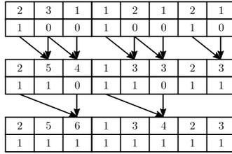
Figure 3.13: Segmented scan applied to an array with three segments. In each step the top row holds values and the bottom row holds the segment head flags.
