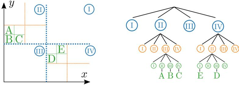
Figure 3.8: Left: Spatial partitioning of a quadtree. Right: Corresponding tree.
