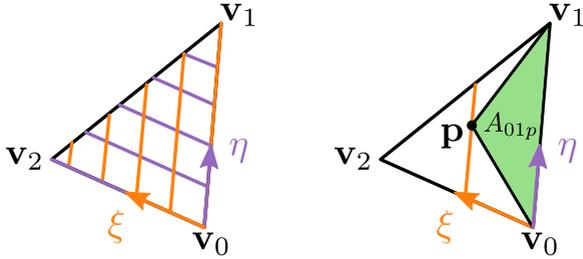
Figure 6.8: Iso lines of barycentric coordinates (left) and computation of barycentric coordinates of a point  $\mathbf{p}$  in the triangle plane (right).
