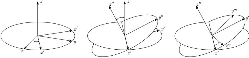
Figure 3.1: Euler angles with rotation order z-x-z applied to the coordinate axis in sequence from left to right.
