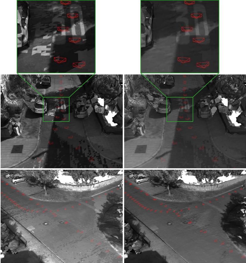
Figure 7.7: Comparison of textured reconstruction with raw images (left) and with images corrected for exposure and vignetting (right). The horizontal change of brightness in the top images is caused by a house casting a shadow onto the street. In the example at the bottom, it can be seen how isolated triangles vanish, as does the sudden change of brightness on the street to the right.
