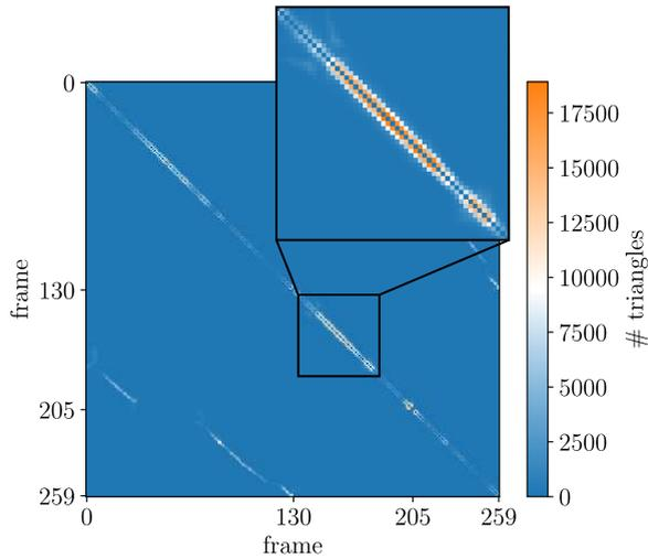
Figure 7.8: Number of observed triangles by pairs of cameras. Frames 0-129, 130-204 and 205-259 are sequences, each. Entries off the main diagonal show the coupling between the sequences. The enlarged area shows an area which is covered by one of the sequences only. Therefore, most residuals are between triangles of consecutive frames.
