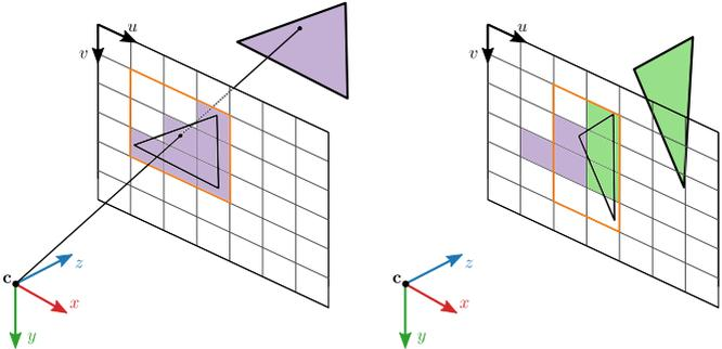
Figure 6.1: Rasterizing two triangles. A ray is shot through each pixel within the orange rectangle which is the enclosing bounding box of the triangle's projection. The green triangle is closer than the purple triangle. Therefore, the depth buffer and index buffer is overwritten with the new values.
