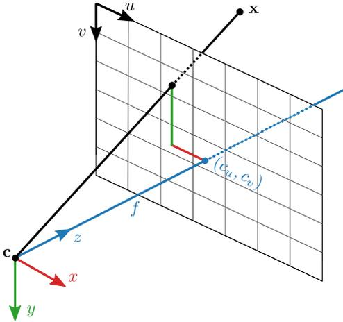
Figure 4.2: Pinhole model used for depth from stereo.
