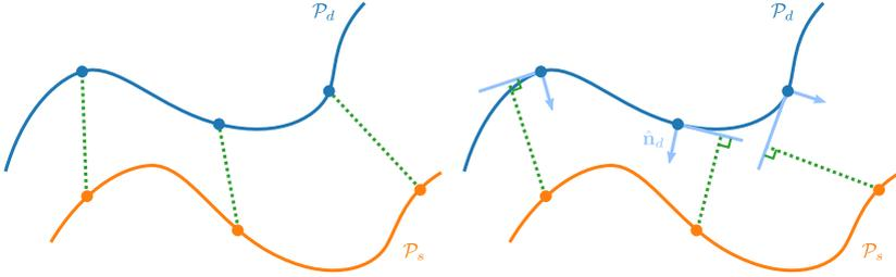
Figure 3.19: Costs of point-to-point (left) and point-to-plane ICP (right). The sum of squared lengths of the dashed green lines is minimized.
