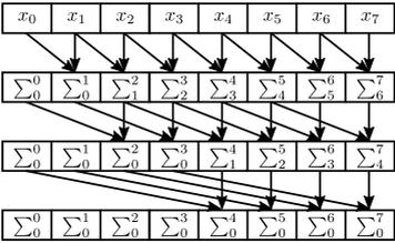
Figure 3.12: Computation steps for an inclusive scan for an array with eight elements. After three steps the array holds the cumulative sum of its input data.
