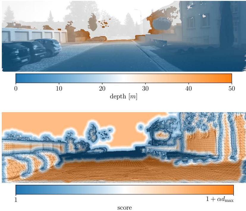
Figure 6.3: Camera image with overlaid depth map (top) and reconstructed mesh with overlaid scores for each pixel (bottom). Areas without depth discontinuities, like road and walls, have a high score whereas areas close to depth discontinuities, like around the parked cars on the left hand side or the tree on the right, have a low score which makes it unlikely that image information from these pixels will be used for texturing.
