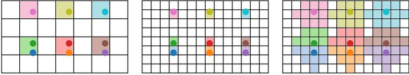
Figure 4.6: Point measurements (colored circles) are assigned to pixels of three sensor models. The last sensor model uses point splatting which assigns a single measurement to multiple pixels (boxes with light shading).
