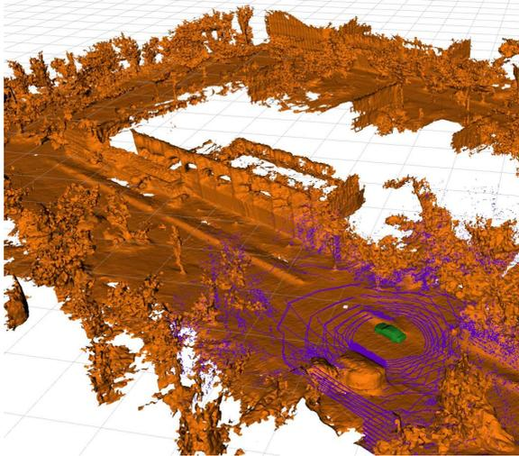
Figure 8.4: Live visualization of the localization map (orange) and current estimate of Bertha’s pose (green vehicle model). The current point cloud from LiDARs is shown in purple.
