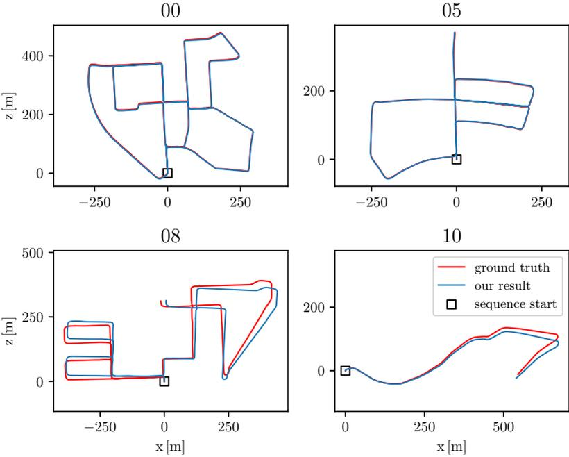
Figure 7.1: Trajectories of KITTI odometry benchmark sequences 00, 05, 08 and 10 using our method (blue) and ground truth (red).
