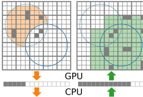
Figure 4.5: Visualization of the streaming process. The visible area of a sensor moves from dashed to the solid circle. Gray boxes represent allocated voxels. The bold lines represent voxel blocks. All voxels within the orange area are streamed out while all voxels within the green area are streamed in. Streaming is done by first moving data to a buffer and then from the buffer to its destination.
