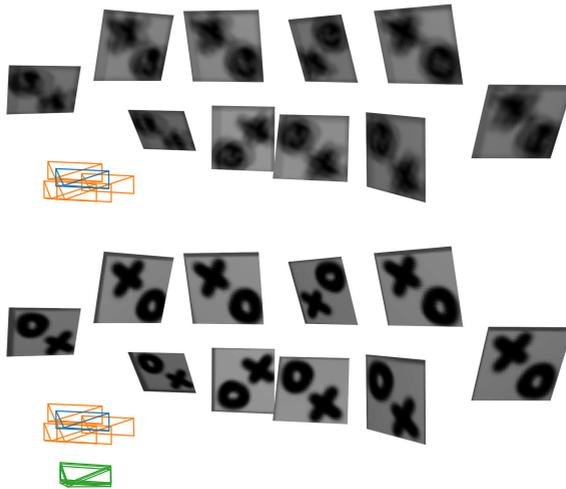
Figure 6.11: Initial camera poses with texturing result (top) and after camera pose optimization (bottom). The orange sensor frames are the initial frames, the green ones are after optimization and the blue ones are the ground truth. The gray borders along the top and left edges of the squares come from texturing with the background color which is a dark gray.
