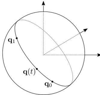
Figure 3.2: Visualization of what SLERP would look like in 3D for  $\mathbf{q}(t) = \text{slerp}(t, \mathbf{q}_0, \mathbf{q}_1)$ . Actual SLERP interpolates on a 4D sphere.
