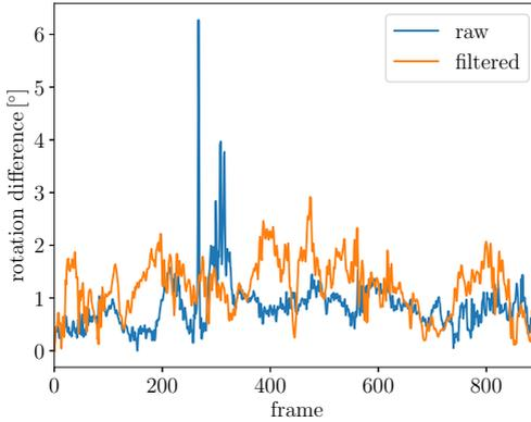
Figure 8.3: Rotation differences between visual localization and LiDAR localization.
