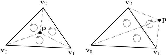
Figure 6.2: Winding of triangles when one vertex is replaced by point  $\mathbf{p}$ . On the right hand side it can be seen that the triangle  $\mathbf{p}, \mathbf{v}_1, \mathbf{v}_2$  has a clockwise winding, as opposed to the other two triangles.
