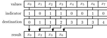
Figure 3.14: Compaction operation on an array. In the final array only the elements with an indicator of one are present.
