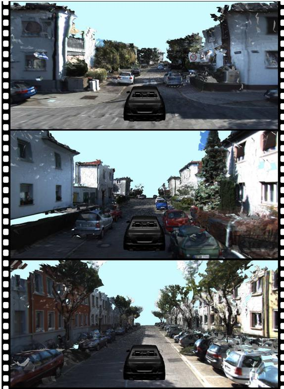
Figure 8.5: A virtual model of Bertha follows a trajectory in simulation. Actual vehicle dynamics are simulated using a game engine.
