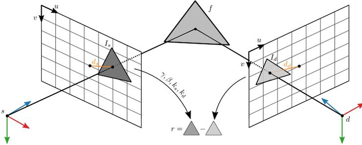
Figure 6.10: Visualization of residual computation between two cameras which see the same triangle. The brightness of the triangle in the source camera is mapped to the destination camera using the estimates of  $\gamma, \beta, k_s$  and  $k_d$ . The remaining brightness difference is the residual.
