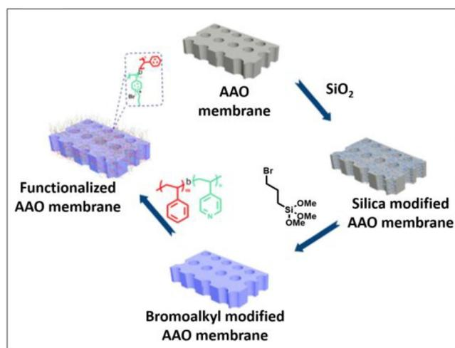
**Fig. 3** Schematic illustrating of grafting to strategy for preparing poly(styrene)-*block*-poly(4-vinylpyridine)/AAO composites. Reprinted with permission from ref. [33]. Copyright 2018 Elsevier
