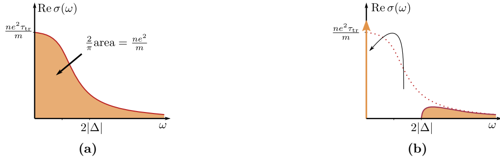
Figure 1.2: (a) shows the Drude peak (1.11) of the optical conductivity of a metal. (b) illustrates the spectral weight transfer as the system becomes a superconductor. Due to the f-sum rule (1.9), the spectral weight is conserved, and the gapped part ( \omega < 2|\Delta| ) is transferred into the weight of the delta function which is responsible for the zero resistivity.
