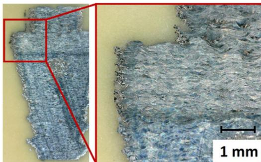
**Figure 2.** Sample shown as cut, embedded, polished and etched. Different material compositions visible for the lower and top part.
