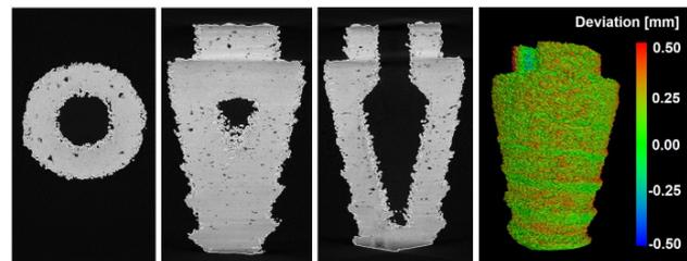
**Figure 3.** X-Ray CT scan of the implant specimen showing X, Y and Z cross section projections and part deviation plot from the nominal CAD model.
