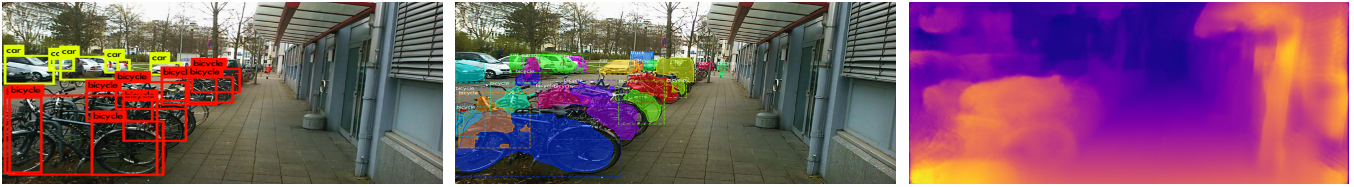
Figure 2: Computer vision module: object detection (YOLO [46], left), instance segmentation (Mask-RCNN [15], center), and depth estimation (MonoDepth [27], right) of an image captured by our camera.
