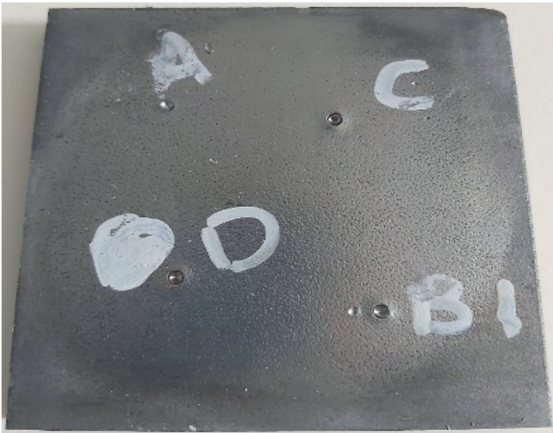
Figure 91: Upper surface of investigated specimen of S355 and the craters for the four impacts
