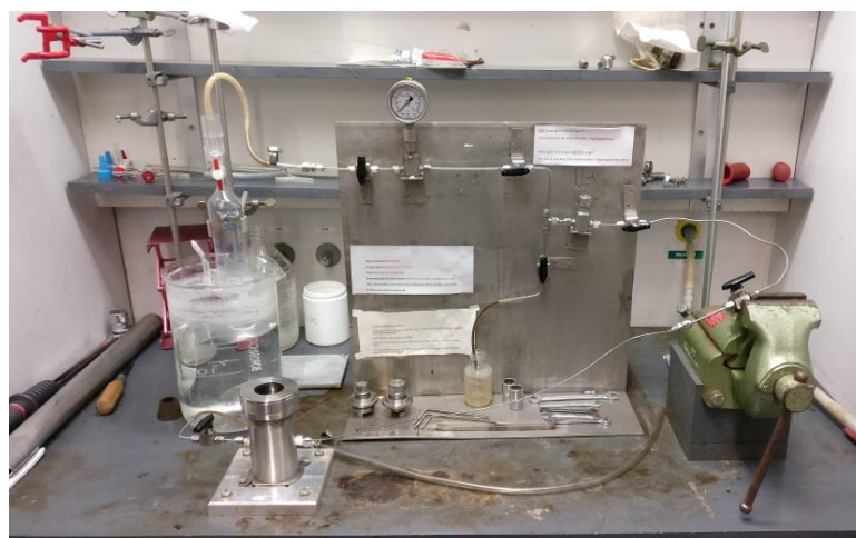
Figure 3-3 Gas collection system
