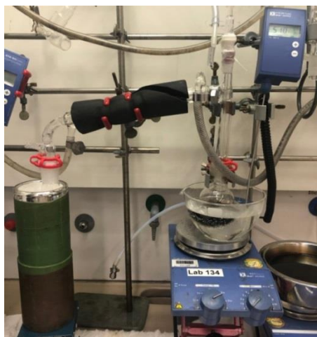
Figure 5-2 Controlled evaporation system to collect evaporated solvents with volatiles
