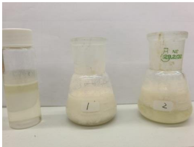
Figure 6-3 Mixed samples from HTL of palmitic acid and lysine at 250 °C
