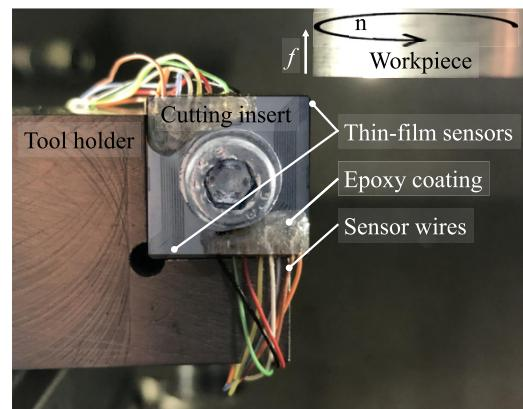
**Figure 9:** Cutting process setup using in-tool integrated thin-film temperature sensor.
