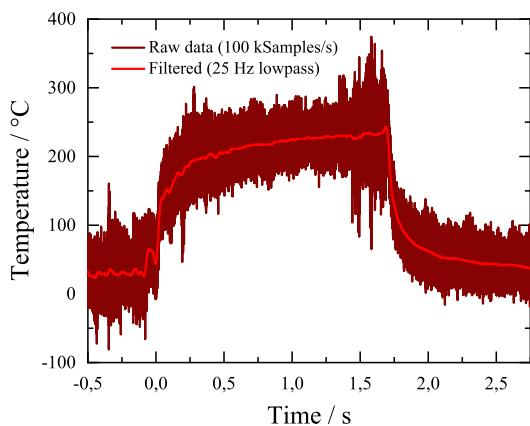
Figure 10: Measured tool-chip interface temperature.
