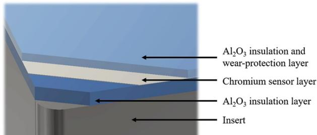
**Figure 1:** Layer materials of the thin-film systems.
