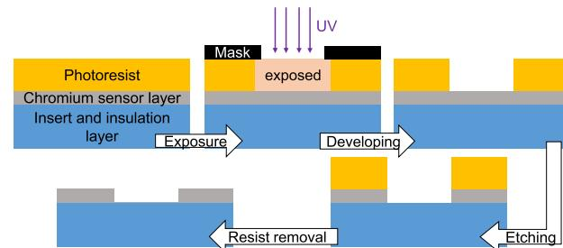
**Figure 6:** Structuring process diagram.
