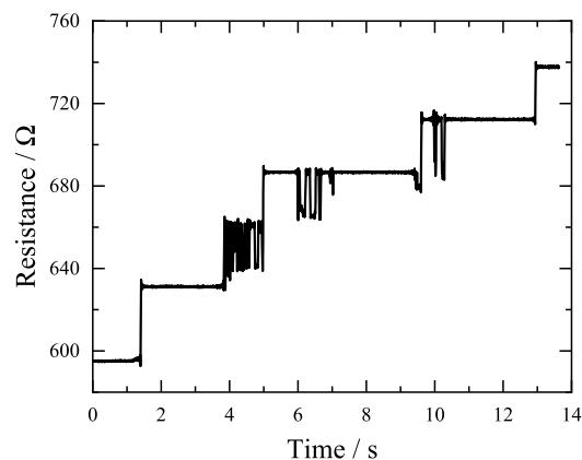
Figure 11: Demonstration of the working principle of wear measurements obtained in a laboratory experiment.
