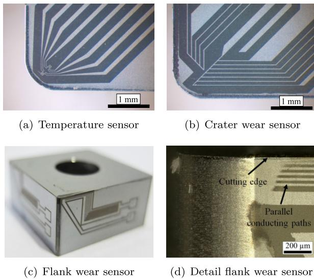
**Figure 7:** Thin-film sensors on cutting tool rake and flank face.
