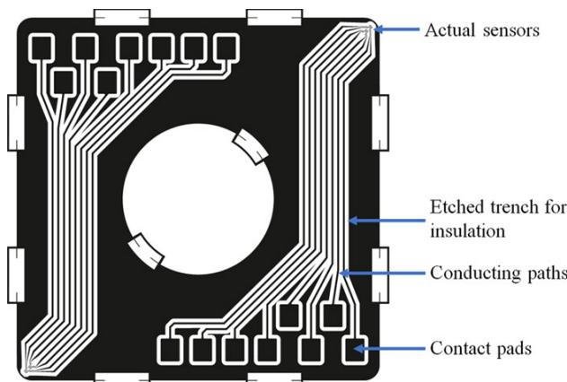
**Figure 2:** Temperature sensor design.
