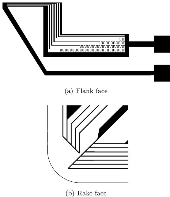
**Figure 5:** Wear sensor design for flank and crater wear monitoring.
