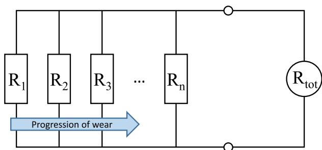
**Figure 4:** Circuit diagram of wear sensors.
