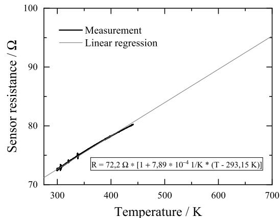
**Figure 8:** Thermoresistive characteristic curve.
