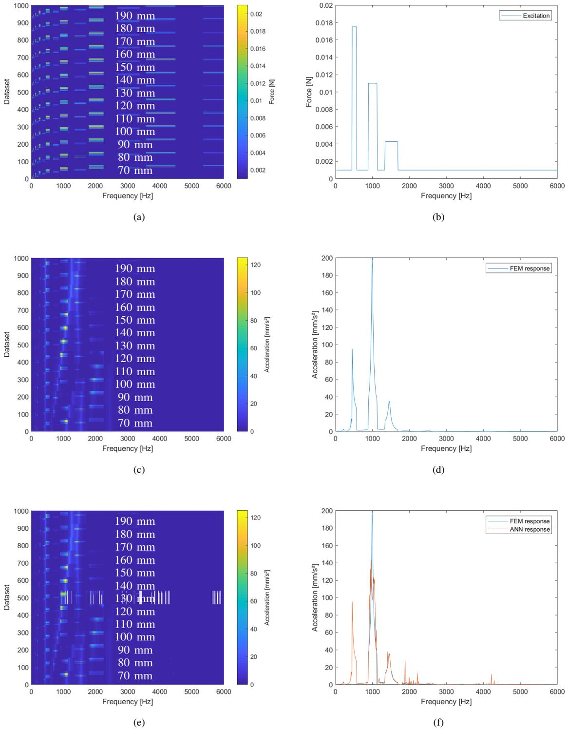
Figure 5. (a) Applied excitation for all structural configurations and force amplitudes. Increase of the  $x$ -value after each 77 datasets. (b) Force spectrum of dataset 512 which is related to a  $x$ -value of 130 mm. (c) Calculated FEM-response for all structural configurations and force amplitudes. (d) Acceleration spectrum of dataset 512 which is related to a  $x$ -value of 130 mm. (e) ANN response spectrum for all datasets. (f) Comparison FEM-response and ANN-response for dataset 512.
