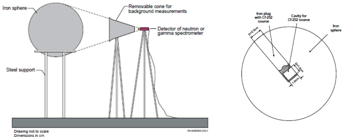
Fig. 1.1. The lay-out of the IPPE experiment (left) and arrangement of the iron sphere with cavity for  $^{252}\text{Cf}$  source closed by the iron plug (right) [19 - 23].
