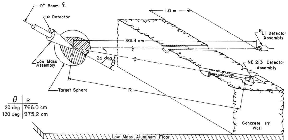
Fig. 1.4. The lay-out of the LLL experiment for with iron spheres and pulsed D-T neutron source [4].
