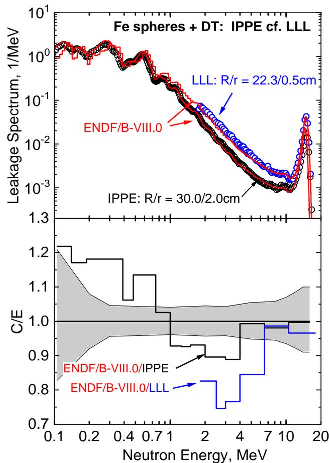
Fig. 1.6. Comparison of the spectra of neutrons leaking from Fe sphere fed by pulsed D-T neutron source: measurements - LLL sphere of outer radius 22.3 cm (4.8 mfp) [4, 5] and IPPE sphere of radius 30 cm [35]; calculations - MCNP with ENDF/B-VIII.0. Bottom part shows the C/E ratios obtained from integration in the selected energy intervals.
