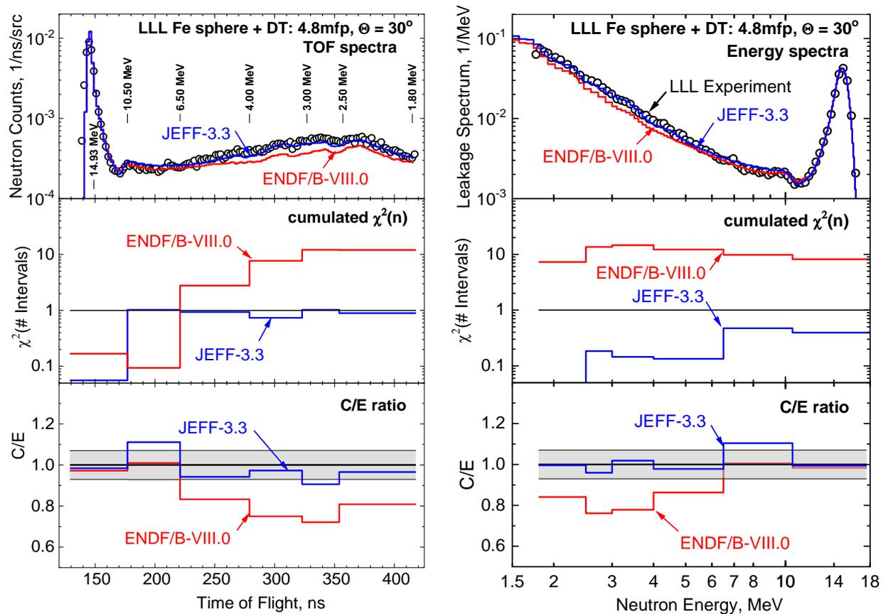
Fig. 5.2. The TOF (left) and energy (right) neutron leakage spectra for the LLL iron sphere with wall thickness 4.8 mfp ( $\varnothing 44.6$  cm) pulsed by the D-T source and measured at angle  $30^\circ$ : open circle - experiment [4], curves - MCNP simulation with nuclear data from ENDF/B-VIII.0 (red) and JEFF-3.3 (blue). Upper part of figures – energy spectra, middle –  $\chi^2$  cumulated over  $n$  integration intervals, bottom – C/E for these intervals.
