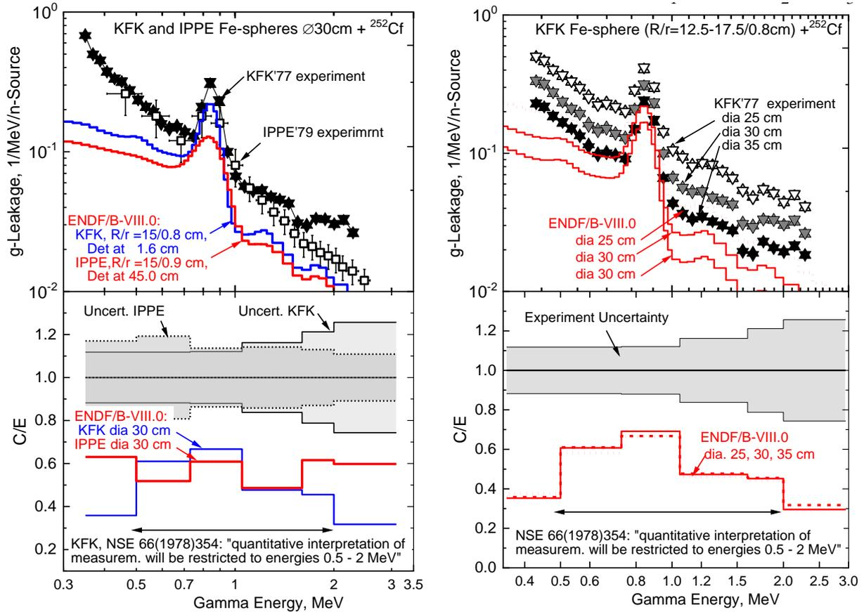
Fig. 1.3. Comparison of the spectra of  $\gamma$ -rays leaking from Fe sphere fed by the  $^{252}\text{Cf}$  source: KFK vs. the IPPE measurements for sphere  $\text{Ø}30\text{ cm}$  (left) and all KFK spheres of  $\text{Ø}25 - 35\text{ cm}$  (right). Symbols – measurements; curves – MCNP transport calculations with ENDF/B-VIII.0. Bottom parts plot corresponding C/E ratios integrated in the energy intervals selected to capture the  $\gamma$ -ray spectra features.
