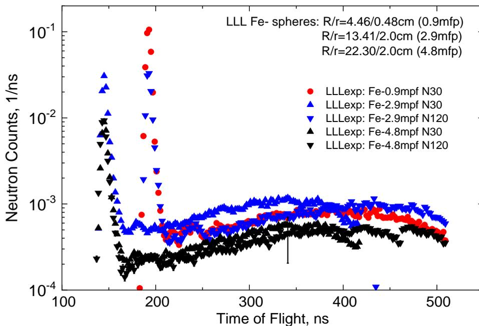
Fig.1.5. The time of flight spectra of neutrons leaking from LLL spheres of different radii fed by a pulsed D-T neutron source and registered by the NE213 scintillation detector positioned at indicated angles.
