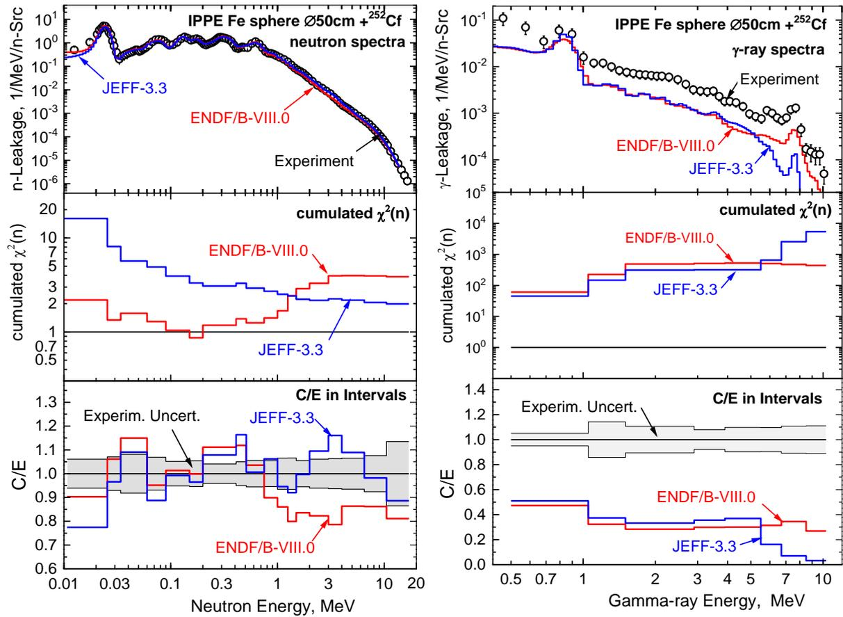
Fig. 5.1. The neutron (left) and  $\gamma$ -ray (right) leakage spectra from the IPPE iron sphere  $\varnothing 50$  cm with  $^{252}\text{Cf}$ (s.f.) source: open circle - experiment [21, 23], curves - MCNP simulation with nuclear data from ENDF/B-VIII.0 (red) and JEFF-3.3 (blue). Upper part of figures – energy spectra, middle –  $\chi^2$  cumulated over  $n$  integration intervals, bottom – C/E for these intervals.
