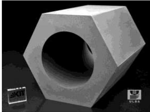
Figure 5: Hexagonal  $\text{TiBe}_{12}$  block after final machining
