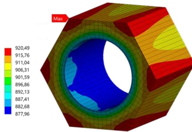
**Figure 3: Temperature distribution within hexagonal  $\text{TiBe}_{12}$  block at the end of a plasma pulse**
