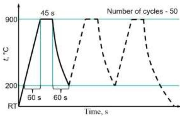
**Figure 6: Change of temperature of  $\text{TiBe}_{12}$  block with time under conditions similar to pulsed operation of the DEMO fusion reactor**
