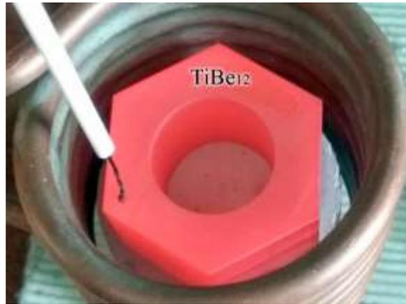
**Figure 7: Induction heating of a  $\text{TiBe}_{12}$  hexagonal mock-up up to 1100 °C as preparation step for advanced thermocycling**
