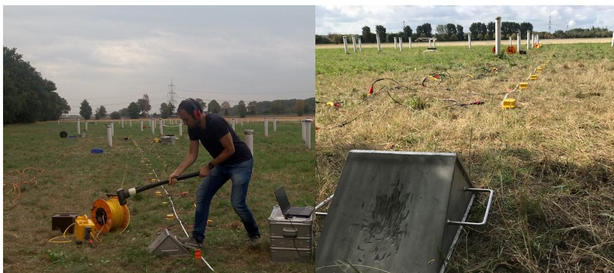
**Figure 7.6:** Overview of the field conditions and the acquisition layout, along with the prismatic source and its operation towards the inline component (direction of the receiver array).
