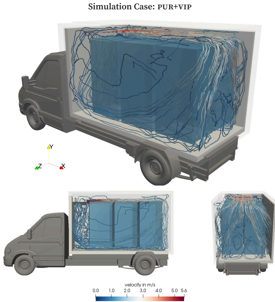
Figure 5.6: Streamline representation of the simulated air flow inside the refrigerated vehicle including surfaces temperatures of the loading for the simulation case PUR+VIP.
