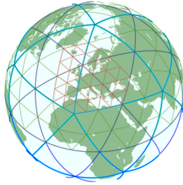
Figure 4.1.: The icosahedral grid of the ICON model. The grid level 0 or icosahedron base grid (light blue lines) has 20 triangular faces, 30 edges and 12 vertices. The first horizontal grid refinement is shown by dark blue lines. The green grid shows the refinement done over the northern hemisphere, and the third one is done over Europe, shown by red lines (Source Giorgetta et al. (2017)).
