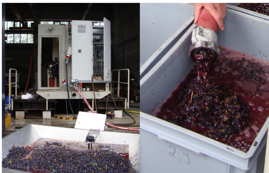
Fig. 2.2.1: Electroporation device with its feeder pump (left) and mash leaving the device (right).
