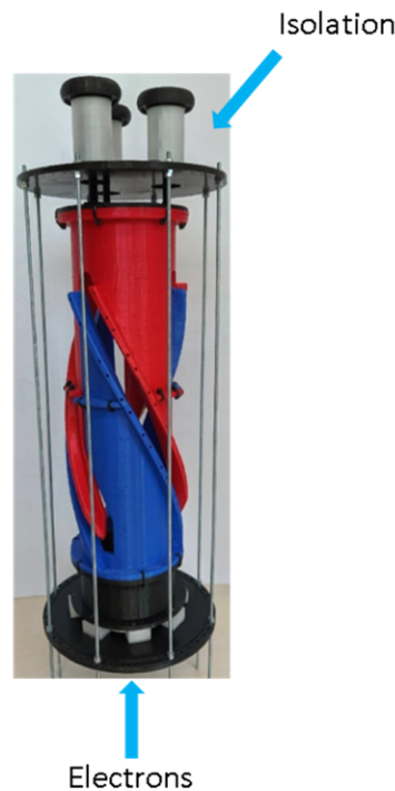
Fig. 1.3.5: 3D print of a 1:4 model of a cylindrical two-stage collector design.
