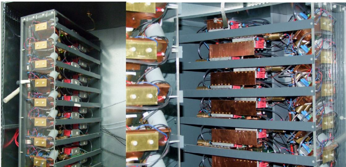
Fig. 2.2.4: 30-stage bipolar pulse generator: Two stacks of 15 stages each mounted inside a shielded enclosure.
