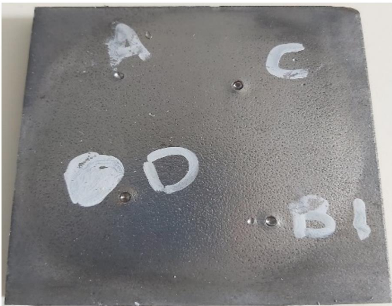
Figure 91: Upper surface of investigated specimen of S355 and the craters for the 4 impacts
