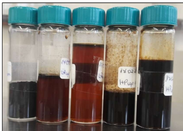
Figure S 3. Upgraded products separated after centrifugation. From the left to the right: spent catalyst after filtration; upgraded aqueous phase and the two last samples in the right side are the upgraded oil.
