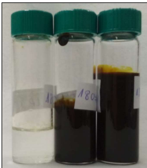
Figure S 4. Products obtained after the second upgrading performed with UBWBO. From the left: upgraded aqueous phase and two bottles containing the upgraded oil.
