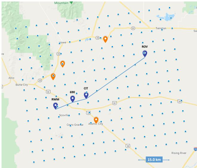
Figure 6.5: NWP grid at the INL Mesonet Region and virtual overhead line. The orange and blue symbols correspond to INL weather stations. The connecting line marks the route of the virtual overhead line. The blue dots represent a portion of the NWP grid, which actually extends to the complete U.S. territory.
