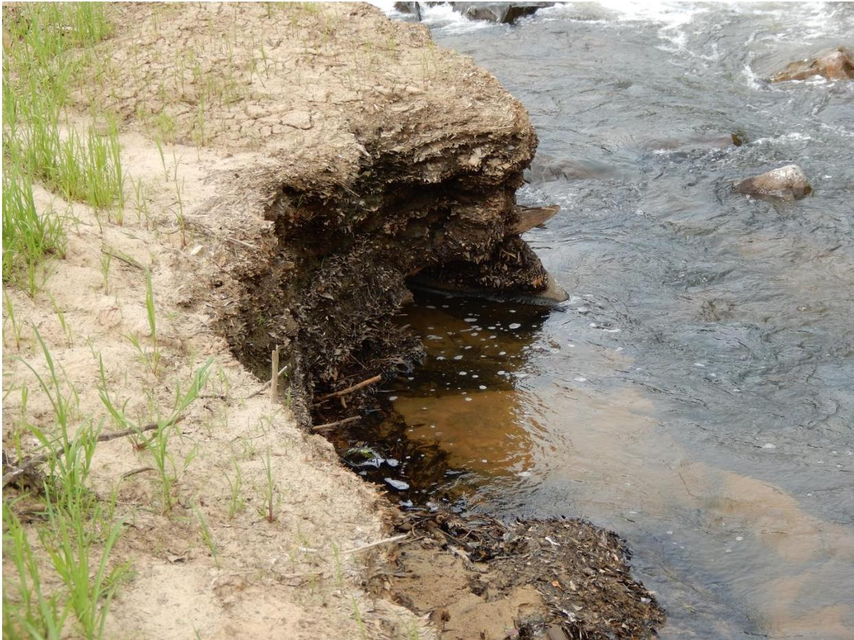
*Figure 8—16. Stratigraphy of the sediment after emptying the Vossoroca reservoir (photo courtesy Stephan Fuchs)*
