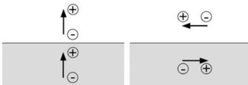
Figure 2.7 : Surface dipole selection rule, dynamic dipole moment perpendicular to the surface (left), parallel to the surface (right) (Figure taken from ref. 100 ).
