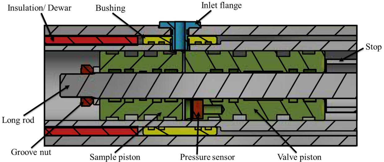
**Figure 4: Construction state-I – probe ready for descent.**
