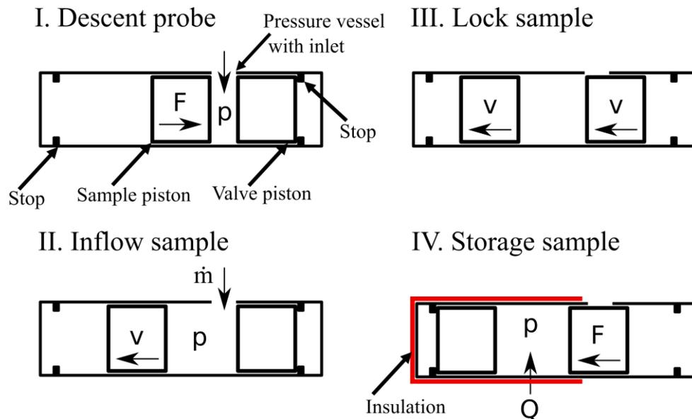
**Figure 1: Schematic design of sample system with states I to IV.**
