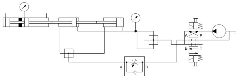
**Figure 3: Schematic fluid sampler: Hydraulic system and pressure vessel with valve piston and sample piston.**
