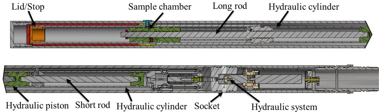
**Figure 2: Construction of fluid sampler functional demonstrator (cut in half-section).**
