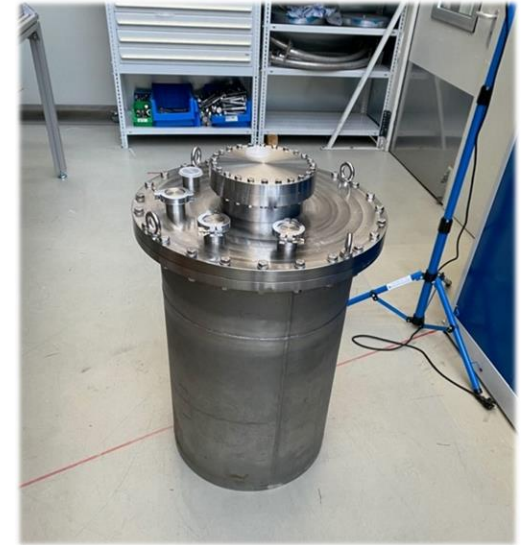
Cryocooler Test Vessel
