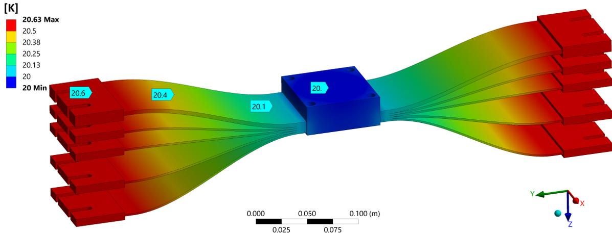
**Fig. 5:** ANSYS® Steady-State Thermal Analysis simulation result for our cold bus out of copper (RRR = 50). We applied a heat load of 6.8 W on the HTS-coil and 20 K cold head temperature.
