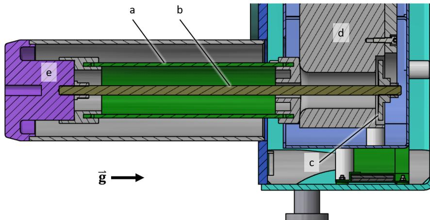
**Fig. 2:** Vertical cryostat cross section including G10-support strut (a), Titanium suspension rod (b), stainless steel support plate (c), HTS-coil steel case (d) and vacuum vessel dome (e) in operational state.
