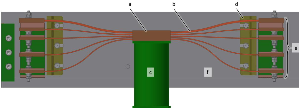
**Fig. 3:** Cold bus installation model front view with cold finger seat (a), flexible copper links (b), cold bus support (c), vibration damper (d), end connection geometry (e) and HTS-coil casing (f).
