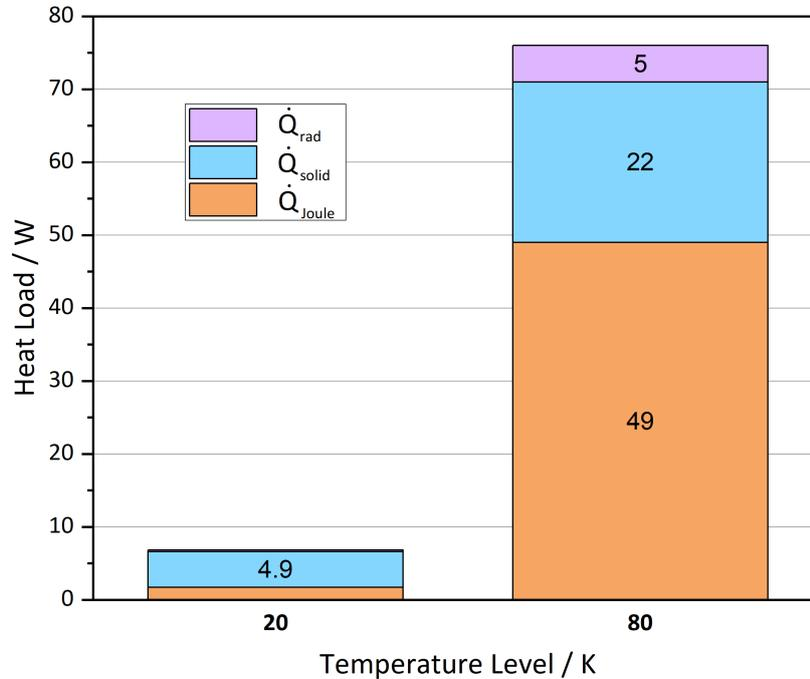
**Fig. 4:** Approximate expected heat loads by type on cryocooler stages at 20 K and 80 K during induction heater operation. Stacked from top to bottom for both temperature levels the contributions to the total heat loads are shown: thermal radiation, heat conduction through solids and Joule heating.
