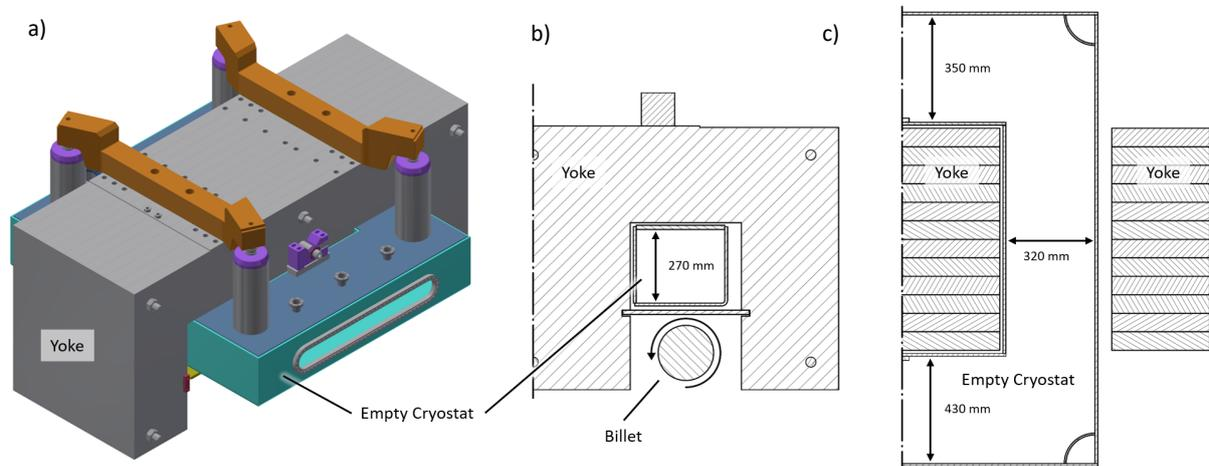
**Fig. 1:** Different yoke and vacuum vessel views: a) 3D-rendered, isometric view, b) one-sided vertical cross section with indicated rotating metal billet, c) one-sided horizontal cross section.
