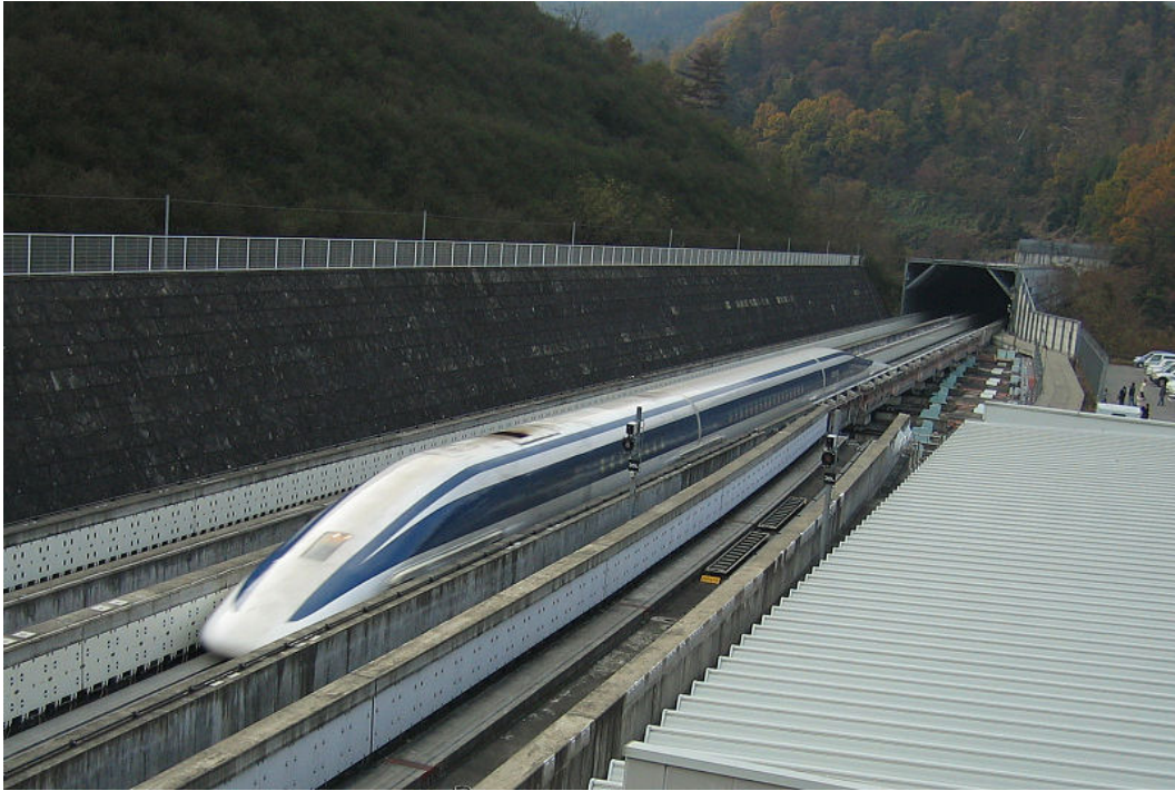
Figure 1.9: Photograph of the JR-Maglev MLX01 on track [41].
