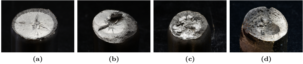
Figure 3.13: Fracture topologies of: a) U20O20 \Delta\sigma_{mic} = 241 MPa; b) U20O17 \Delta\sigma_{mic} = 248 MPa; c) U22O6 \Delta\sigma_{mic} = 459 MPa; d) U22M7 \Delta\sigma_{mic} = 384 MPa
