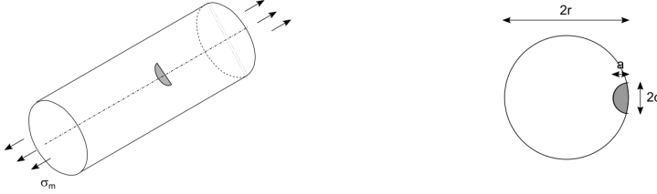
Figure B.3: Cylinder with semi-circular surface crack [161]
