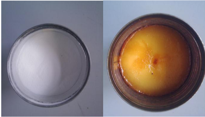
Fig. 4. Left: sample of polyethylene before tests; right: polyethylene sample after tests
