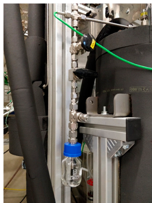
Figure 6. Photograph of the QS site that was installed to avoid gas and liquid back-mixing in the CT. Sampling included the collection of the liquids with the concurrent online-measurement of the gaseous product phase via MS. A minute-scale sampling time was needed to gather enough liquid for analysis.
