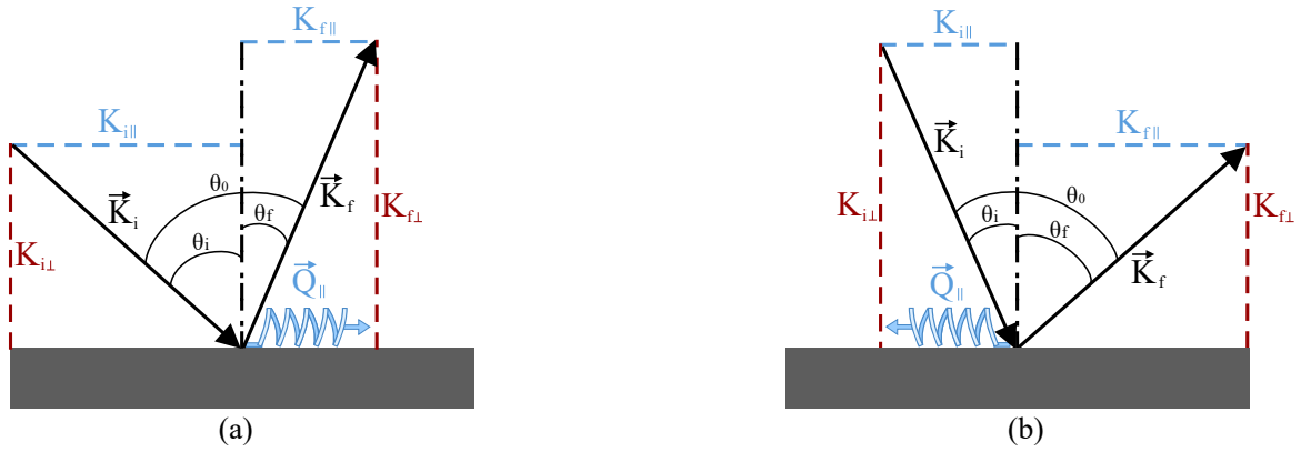
Figure 3.4: A sketch of the scattering geometry in the SPEELS experiment. The incident wave vector of the electron beam and the scattered one is represented by K_i and K_f , respectively. The parallel component of the incident and scattered wave vector is represented by K_{i||} and K_{f||} , respectively.
