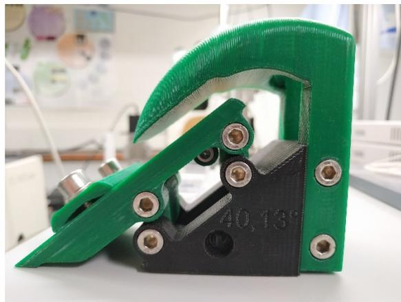
Figure 6.3: The customized fiber polishing tool.
