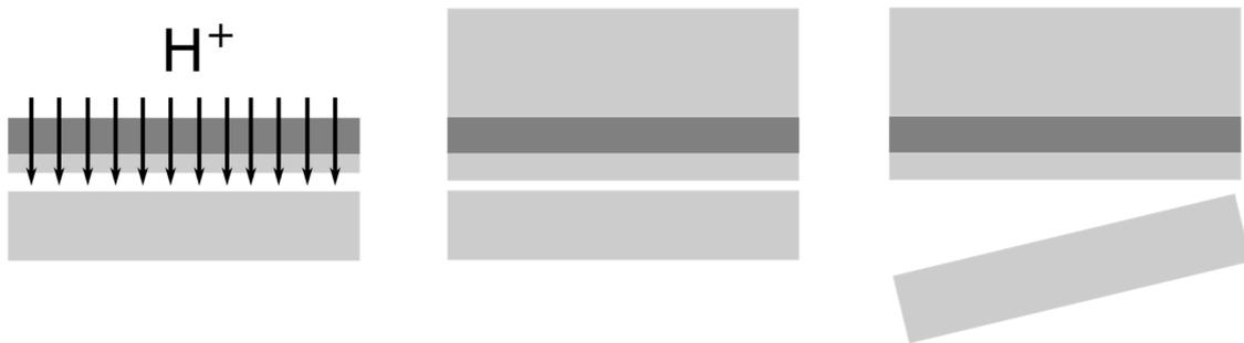
Figure 2.3: SmartCut process: implantation for a thermally oxidized wafer (left), a second wafer is bonded to the implanted wafer similar to the BE method (middle), removal of excess part through thermal processing and subsequent polishing (right).
