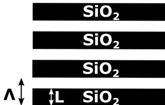
Figure 5.7: Schematic of a reproduction unit in a Bragg reflector.
