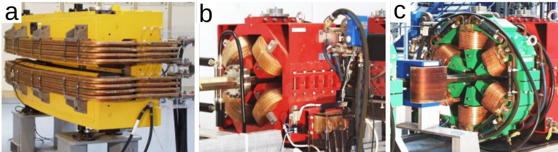
Figure 1.3.: The components of the magnet lattice used at the KIT synchrotron light source. (a) Bending- or dipole magnets which force electrons to travel along a curved path, thereby emitting synchrotron radiation. (b) A focusing quadrupole magnet and (c) a correcting sextupole magnet.
