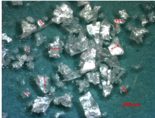
Figure 5.6: Microscope pictures of the PET particles
