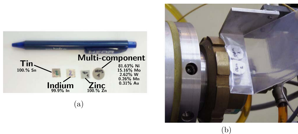
Figure 3. (a) Examples for activation foil samples used in the experiment. (b) The two stacks of activation sample foils in a plastic bag placed on top of the target flange.
