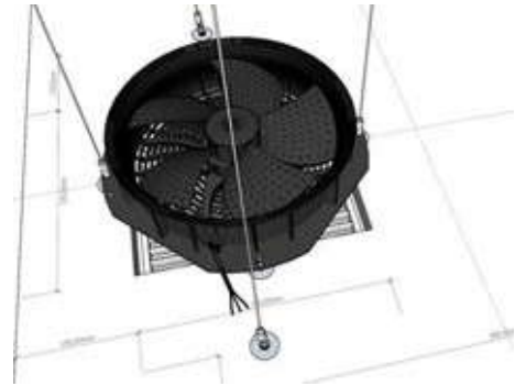
(b) 3D representation from above: fan mounted above hanging panel.
