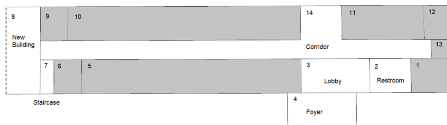
Figure 3. Thermal zones plan on the ground floor. Numbers indicate each thermal zone.
