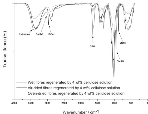
**Figure 4.** IR spectrum of regenerated cellulose fibers after cycle 1, obtained by using a 4 wt% derivative cellulose solution measured directly from ethanol, measured air-dried, and measured after drying in a vacuum oven at 50 °C.
