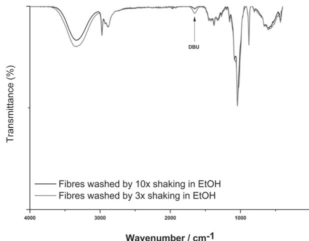
**Figure 5.** IR spectra of regenerated fibers using a 4 wt% derivative cellulose solution in ethanol; IR measurement performed after washing the fibers three times by shaking in ethanol or ten times shaking.
