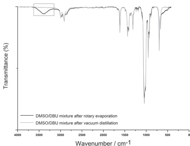
**Figure 3.** IR spectra of a DMSO/DBU mixture after performing a recovery test by vacuum distillation at 90 °C and 20 mbar, compared to a recovery test using a rotary evaporator at 40 °C and below 10 mbar.
