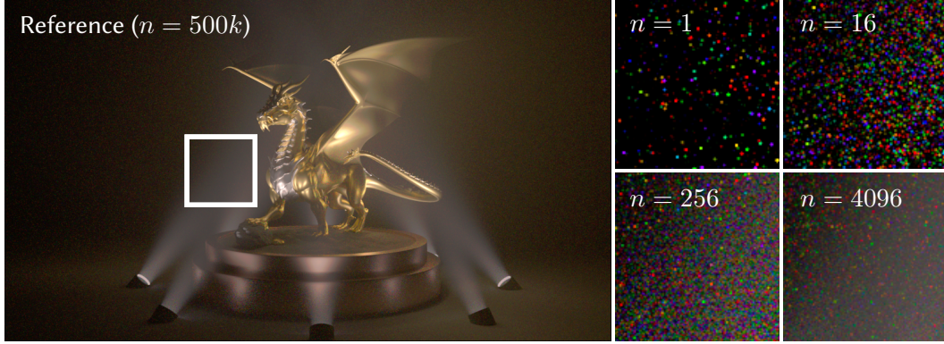
Figure 2.17: Images generated using Monte Carlo rendering exhibit noise due to the variance of the underlying Monte Carlo estimators. This noise vanishes as the number of sampled light paths per pixel n increases. However, if a Monte Carlo sampler cannot sample a complex illumination effect efficiently, the number of paths required to produce a perceptually noise free image can become too large for practical purposes.
