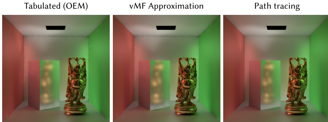
Figure 4.14: Comparison showing only indirect illumination using tabulated emission as octahedron environment maps (OEM) and von Mises-Fisher (vMF) approximation using 5 lobes per color channel for Rich-VPLs and path tracing reference.
