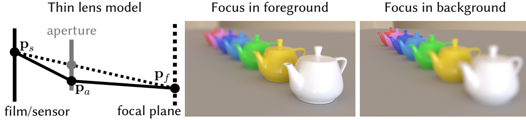
Figure 2.16: The images in this work are rendered using the thin lens camera model, which allows focusing on a specific part of the scene and blurring of others (middle and right). In this model, a ray is generated by sampling a point on the camera’s sensor \mathbf{p}_s and a point on the aperture \mathbf{p}_a . The resulting ray is r = (\mathbf{p}_a, \omega_{\mathbf{p}_a \rightarrow \mathbf{p}_f}) , where \mathbf{p}_f is the intersection of the focal plane and the ray originating at \mathbf{p}_s through the center of the aperture.
