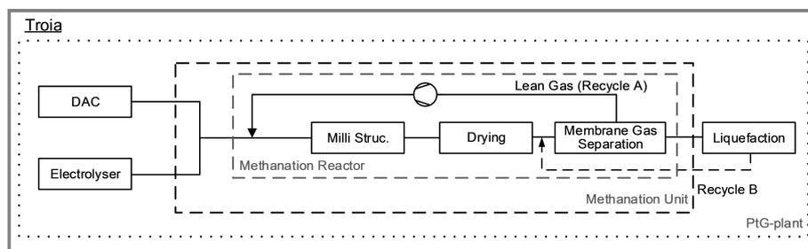
**Figure 4.** Block flow diagrams of the demo site Troia including the chosen system boundaries (dashed lines) for the technical and economic evaluation.
