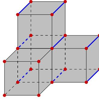
Figure 3.3: The *three-dimensional L-shaped* translation manifold. After the identification (cf. figure 3.1) the translation manifold has a single vertex and six edges (one of which is highlighted). The non-removable singularities consist of the single vertex and the three edges which are all part of the centre cube. The edge singularities have order 3 each (see proposition 3.2.2).
