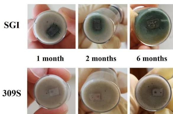
Figure 49. Pictures showing the evolution of steel (top: SGI, bottom: 309S) in contact with bentonite after 1 month (left), 2 months (middle) and 6 months (right).
