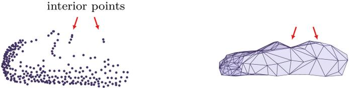
Figure 5.8: Surfel map (left) and triangle mesh (right) reconstruction of an oncoming car. Scan points from the object interior are observed through the windshield *after* the initialization phase and are used to *grow* the mesh, leading to the indicated dent on the roof.
