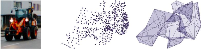
Figure 5.10: Reconstructions of an oncoming bulldozer with highly non-planar surface. The surfel map (middle) is able to represent the object surface reasonably well, whereas the triangulation produces a ragged mesh (right).
