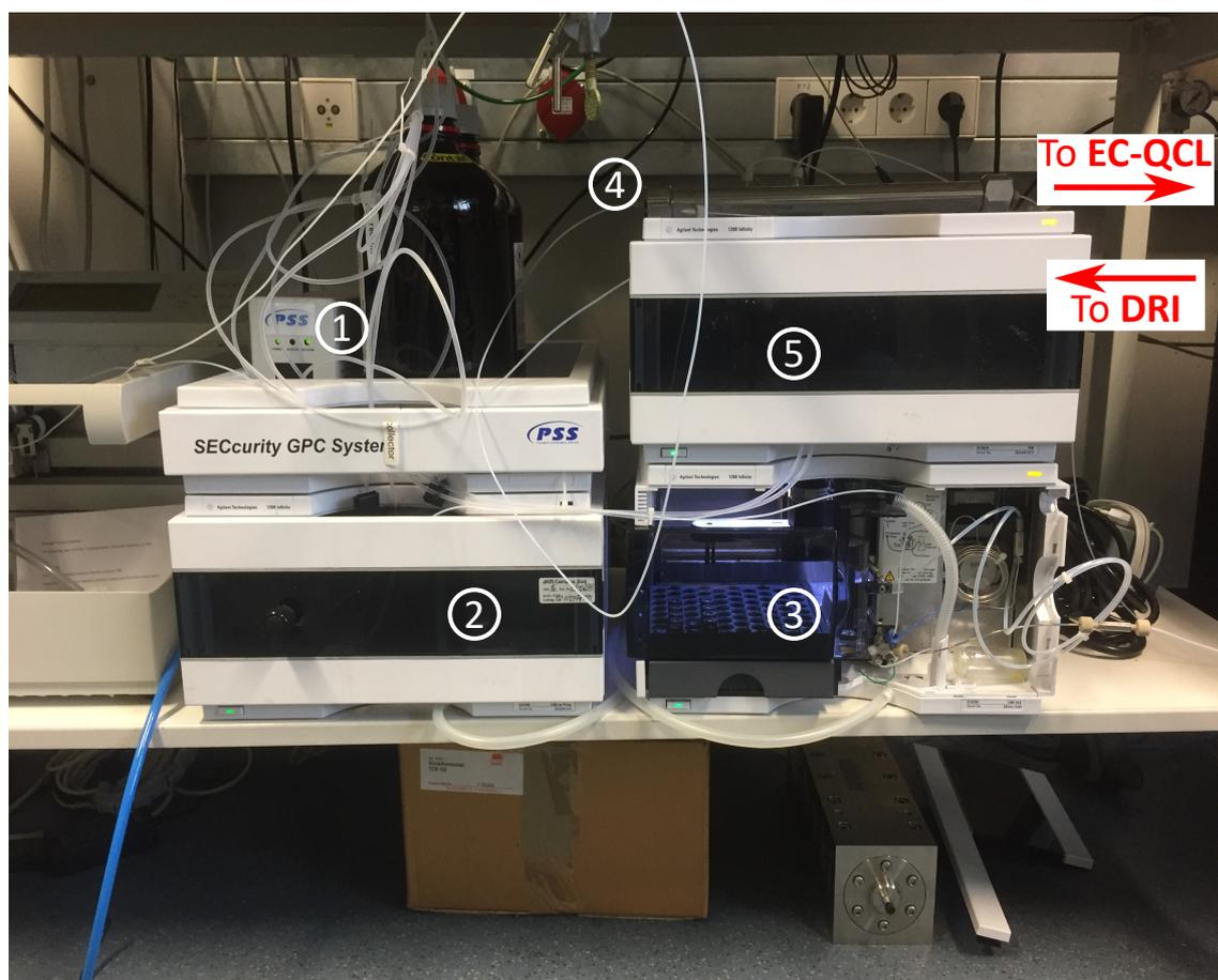
**Figure A.4:** Photograph of the SEC set-up used for hyphenation to the EC-QCL detector. The identification of components labelled in the figure are as follows; (1) external solvent degasser, (2) isocratic pump, (3) auto-sampler, (4) linear M semi-preparative SEC column, and (5) DRI detector. The (red) arrow insets illustrates the analyte flow to the EC-QCL detector after chromatographic separation and then returning to the DRI detector.
