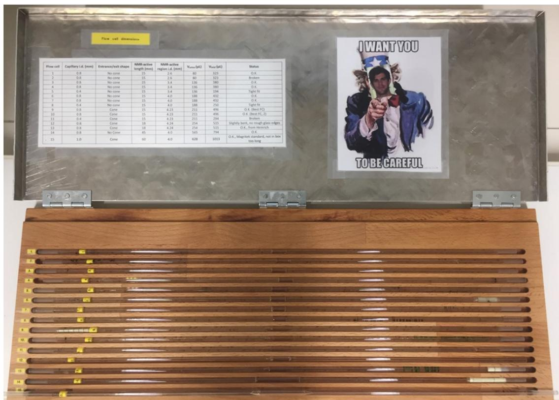
**Figure A.2:** Photograph of the flow cell box and with 15 flow cells inside. Included (the lid) is also a table with a full description of each flow cell, providing information such as flow cell volume, internal capillary diameter and geometry.
