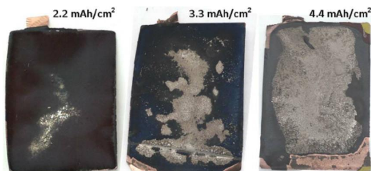
FIGURE 8: IMAGES OF GRAPHITE ELECTRODE AFTER AGEING IN NMC622/GR POUCH CELLS. LITHIUM PLATING APPEARS AS METALLIC DEPOSITS ON THE SURFACE OF THE ELECTRODE. THE FIGURE IS FROM GALLAGHER ET AL. 100
