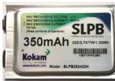
FIGURE 9: A PHOTO OF OUR REFERENCE CELL, 350 MAH HIGH-POWER LITHIUM-ION WITH BLEND CATHODE AND GRAPHITE ANODE.
