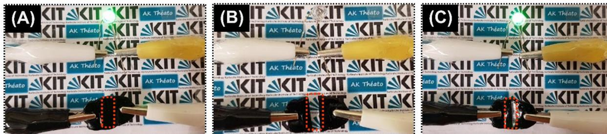
**Figure 4.2.10.** Photographs showing the recovery process of electrical conductivity: (A) hydrogel sample was connected into a circuit powered by an external voltage; (B) hydrogel sample was cut into two separate pieces; (C) the two split pieces was put into contact.
